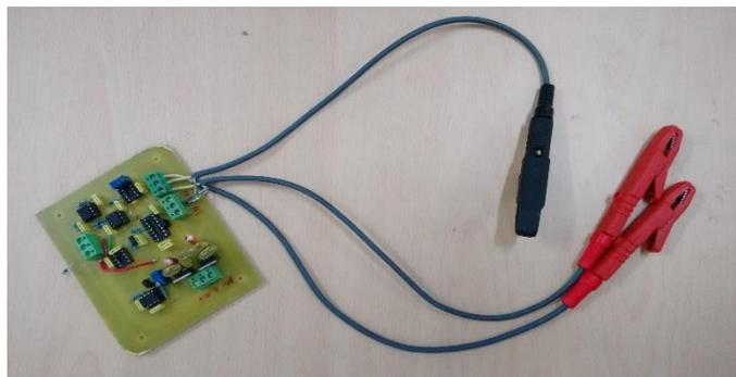
Figure 4.7 Photograph of an I-to-V converter module PCB
