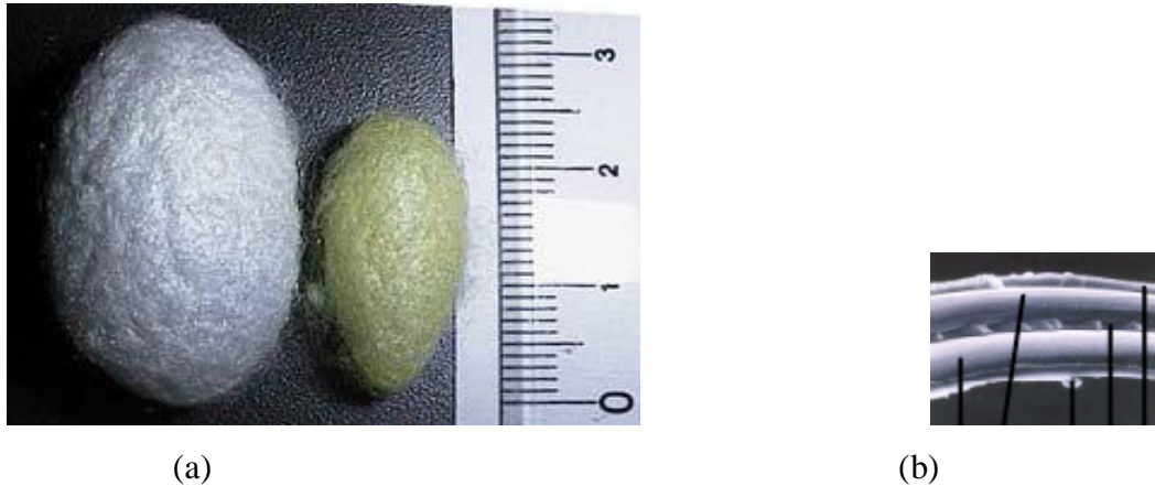
Fig 3.1 Raw Cocoon silks (a) and side view of the silk fibre (b)
