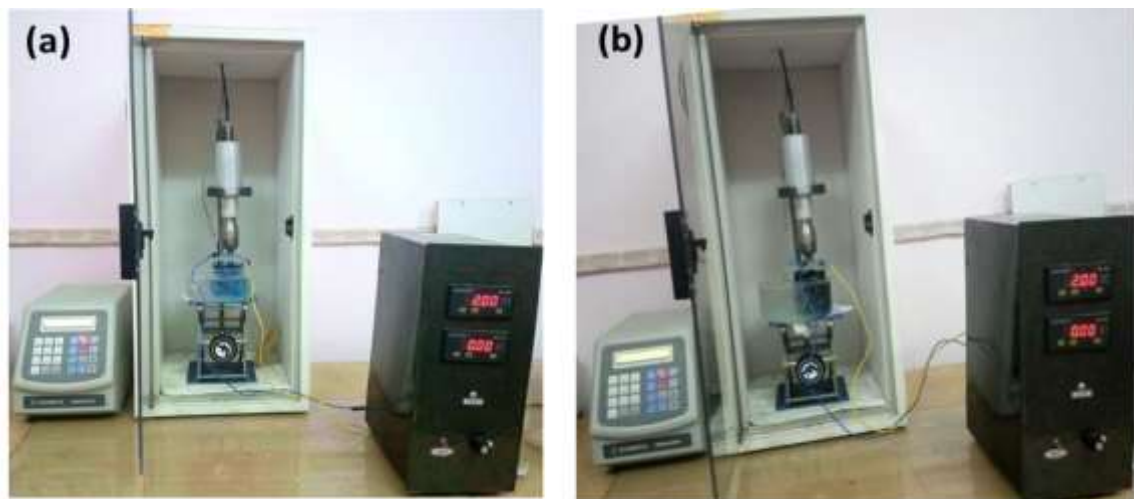
Figure 5.1.1: (a) Experimental setup of pure copper deposition with sonication at a temperature of 15 °C and (b) Experimental setup of copper-FLGPs electrodeposition with sonication
