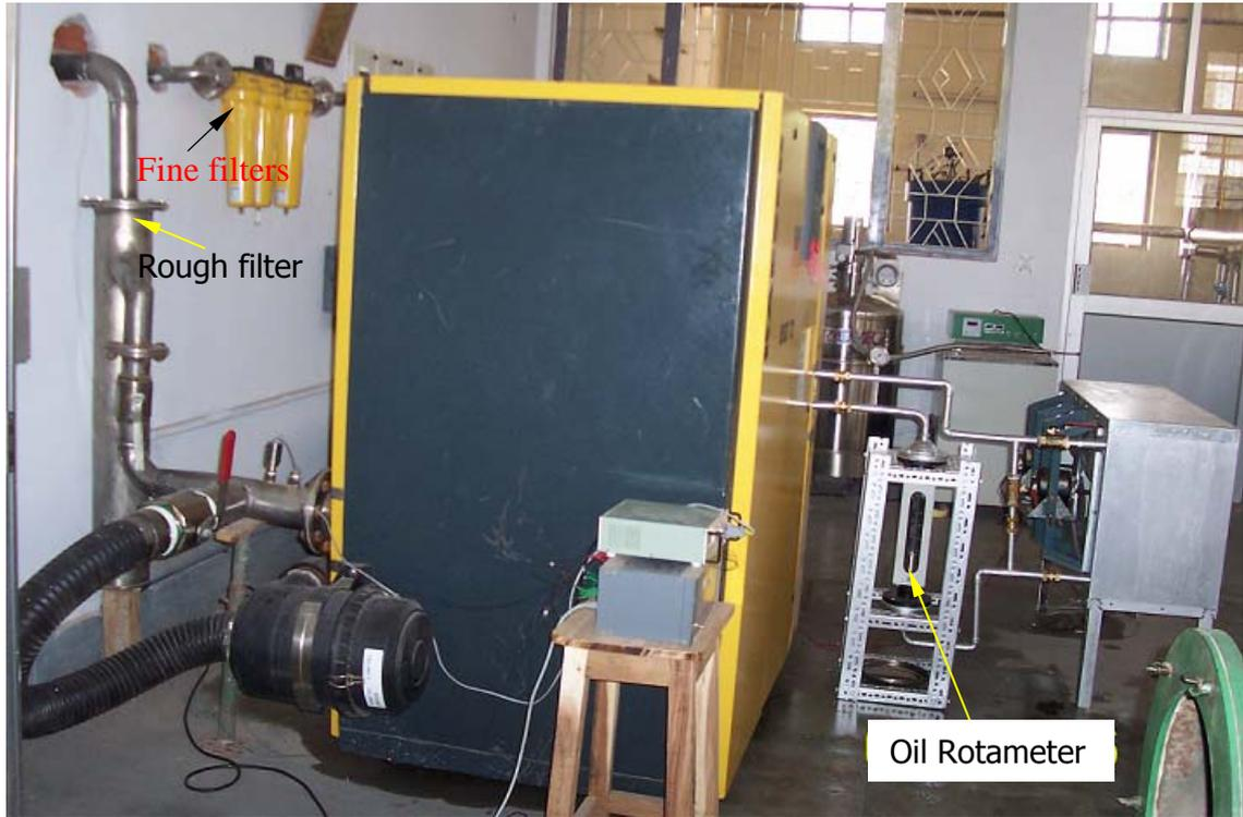
Figure 5.8: Photograph of 37 kW compressor test rig (partial).
