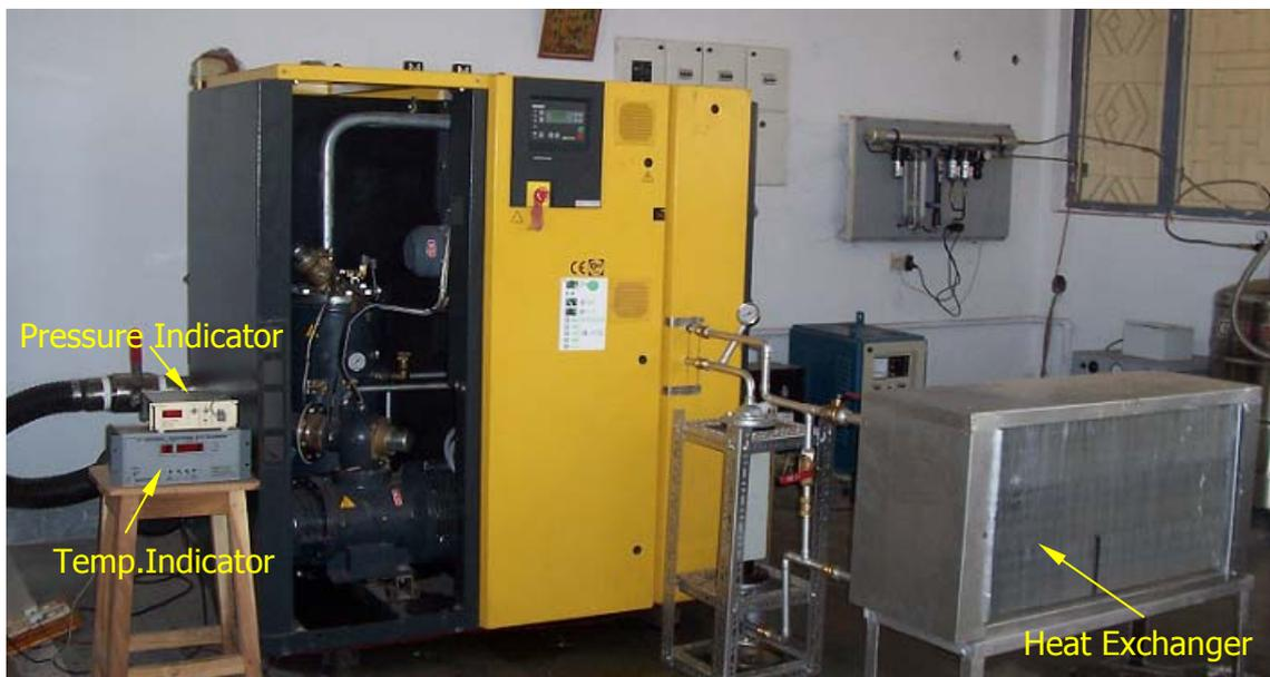
Figure 5.9: Photograph of 37 kW compressor test rig (another view).
