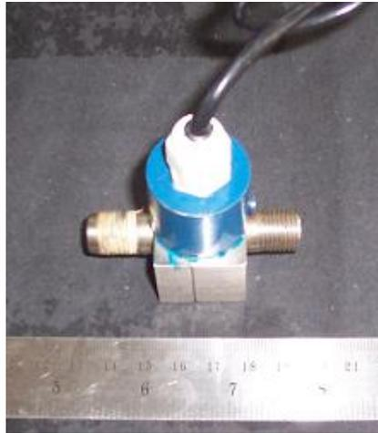
**Figure 5.17:** Photograph of pressure transducer with mechanical fittings.
