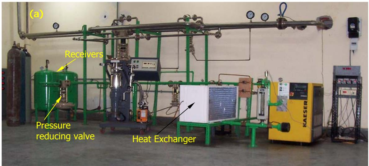
Figure 5.3: Experimental test setup with SM 8 compressor.
