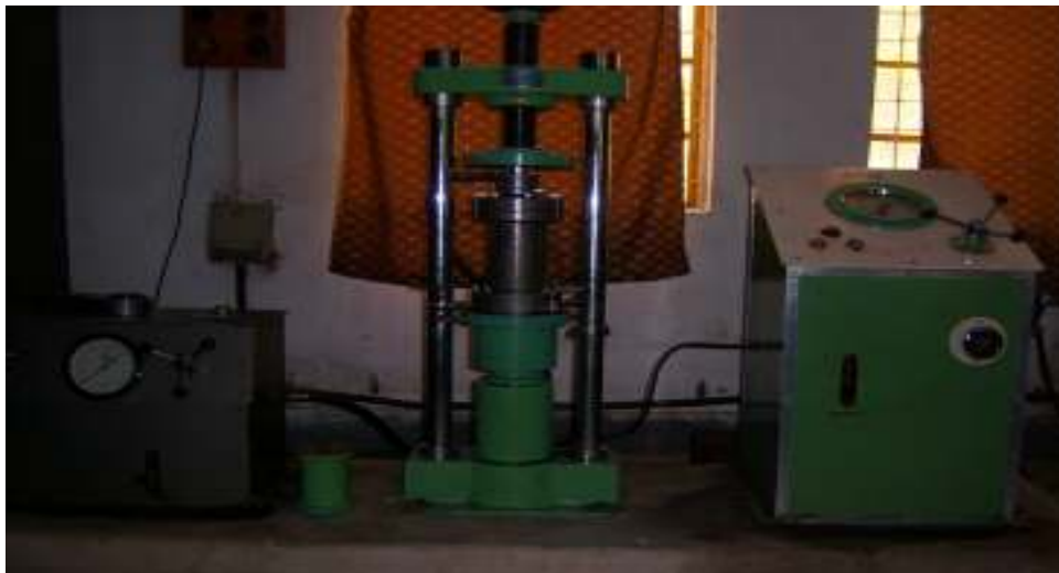
Fig. 4.1 A typical triaxial test apparatus
