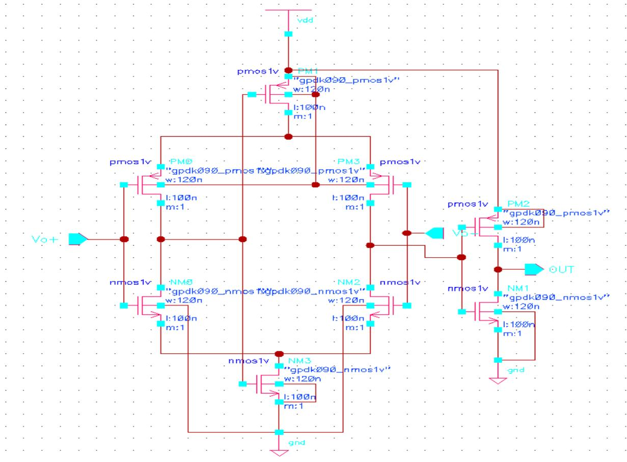
Fig 3.3 Output Buffer Circuit
