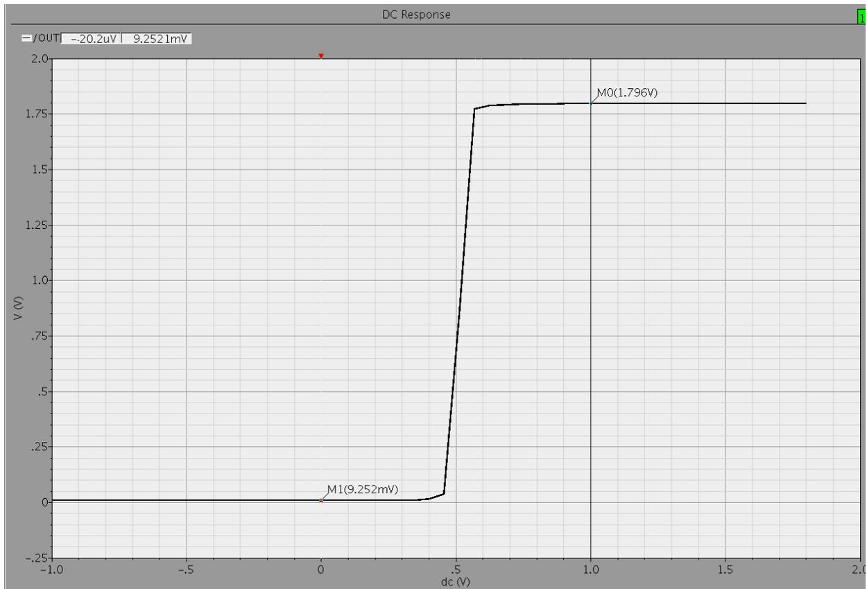
**Fig 3.5 Output Waveform of Comparator and Decision Circuit**
