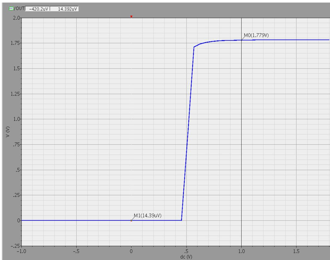
Fig.4.2 .DC analysis of dynamic comparator wave form
