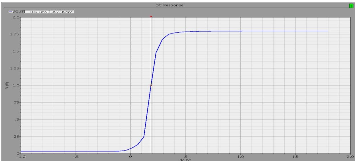
Fig .3.7 Preamplifier comparator offset voltage waveform
