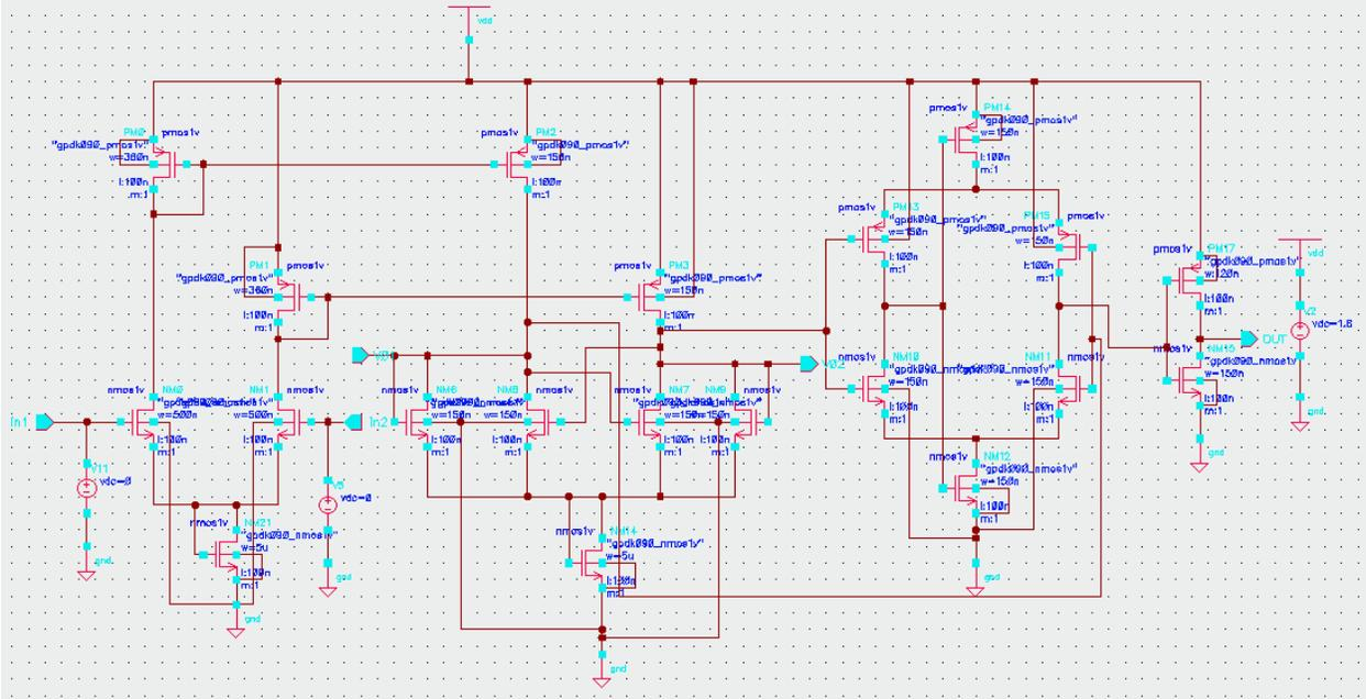
Fig.3.6 Offset circuit for preamplifier based Comparator
