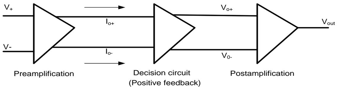
Fig. 2.8 Block diagram of Comparator
