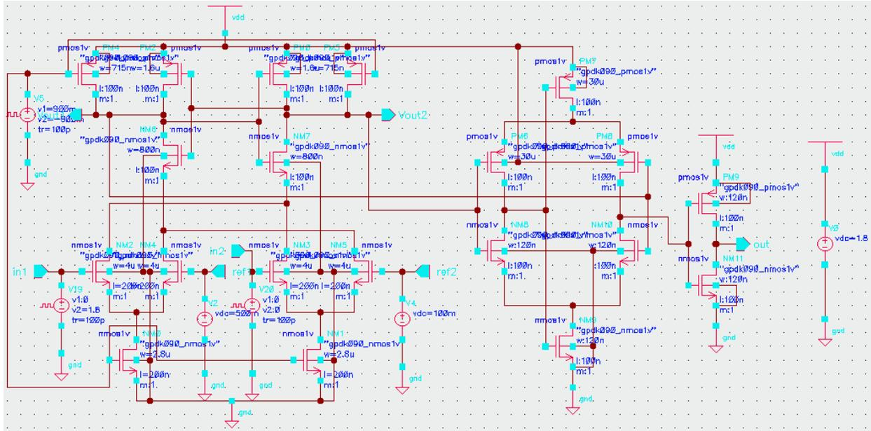
Fig. 3.14 Transient analysis circuit for Differential Dynamic Comparator
