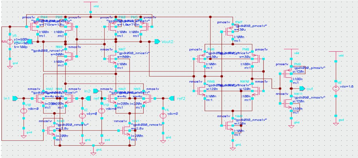
Fig. 3.12 Offset circuit for differential dynamic comparator
