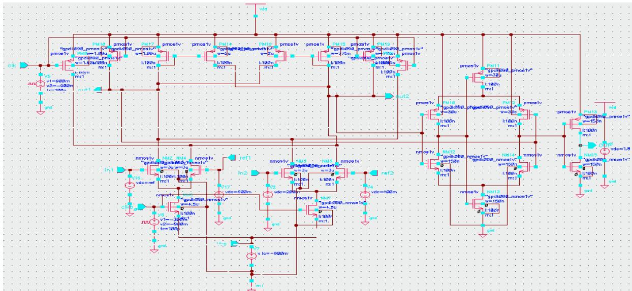
Fig. 4.13 DC Circuit for dynamic comparator PMOS as switch
