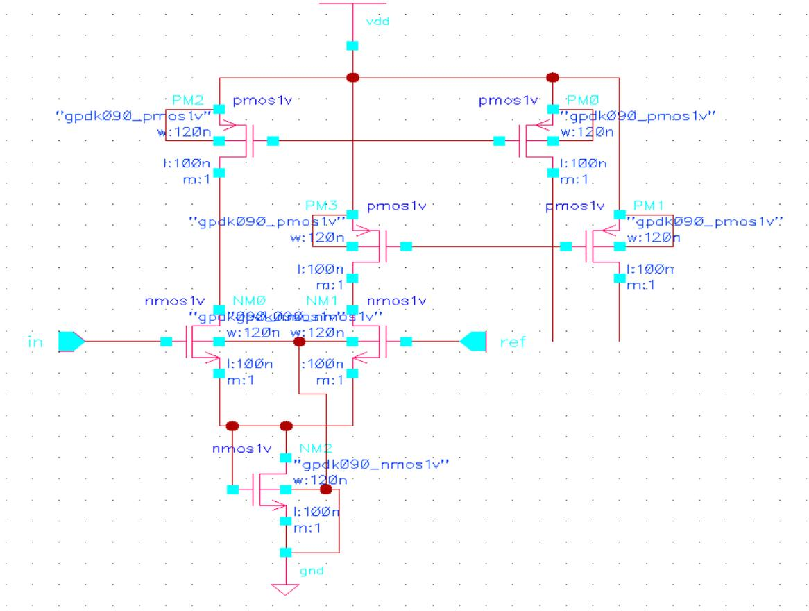
Fig.3.1 Pre-amplification stage of comparator.
