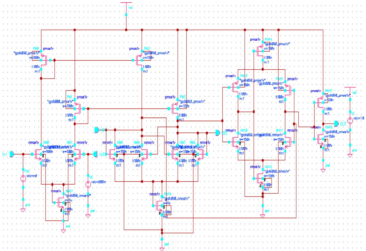
Fig .3.4 Preamplifier based Comparator
