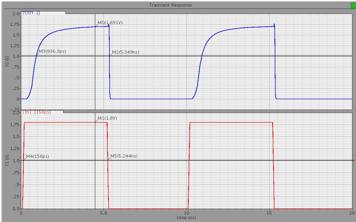
Fig. 4.18 Transient wave form for dynamic comparator PMOS as switch
