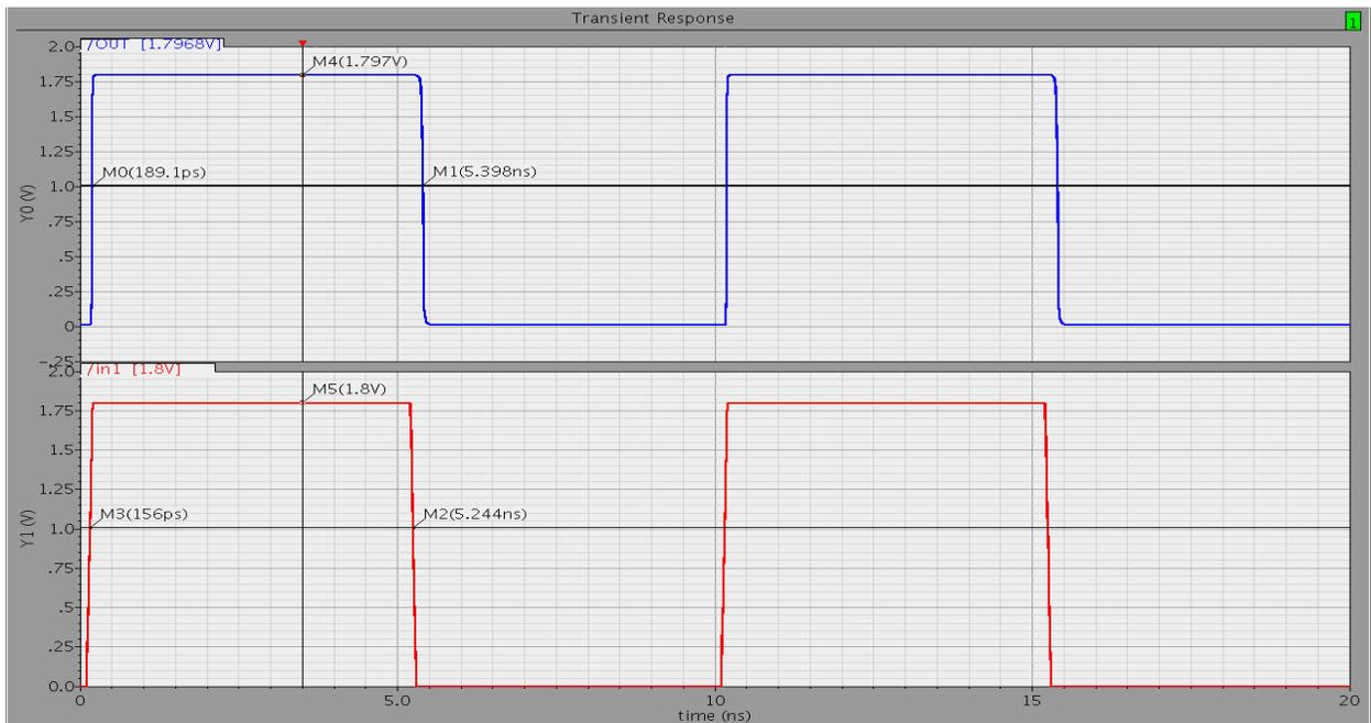
Fig.3.9 Preamplifier based comparator transient analysis waveform
