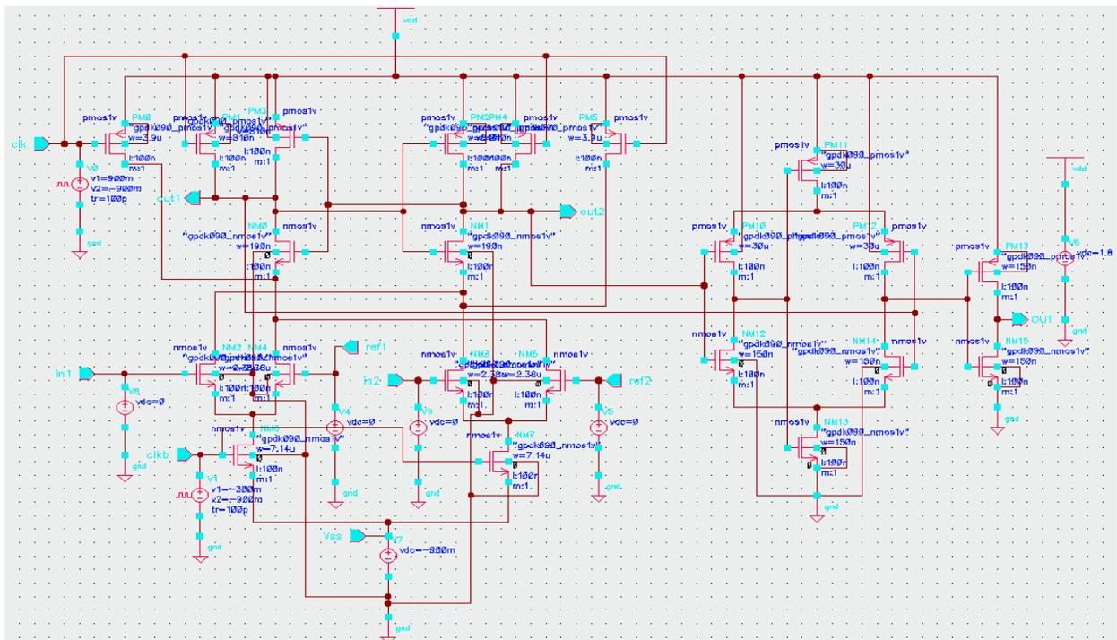
Fig.4.5. Offset voltage circuit for dynamic comparator
