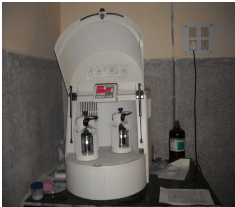
Figure 3.1: Fritsch Pulverisette-5 planetary ball used for mechanical alloying studies.
