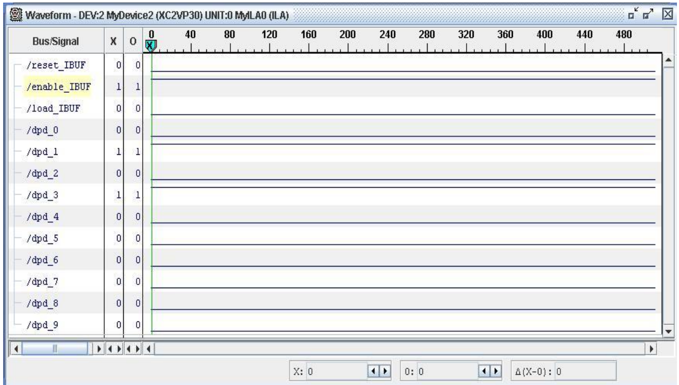
Fig 8. Chipscope result of DPD Encoding decimal number 80.
