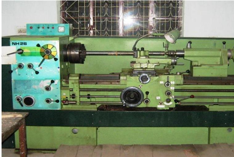
**Fig .4.1 Heavy duty HMT lathe machine**
