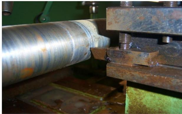
**Fig 4.2 Experimental set up (cutting tool with workpiece)**
