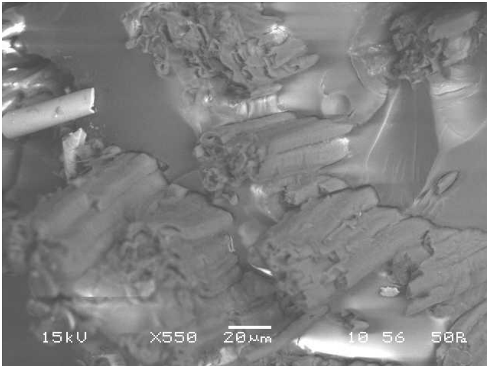
Fig 10(a) and (b). SEM of alkali treated jute fibre composite for 2m/sec and 100 m/sec cross head speed.
