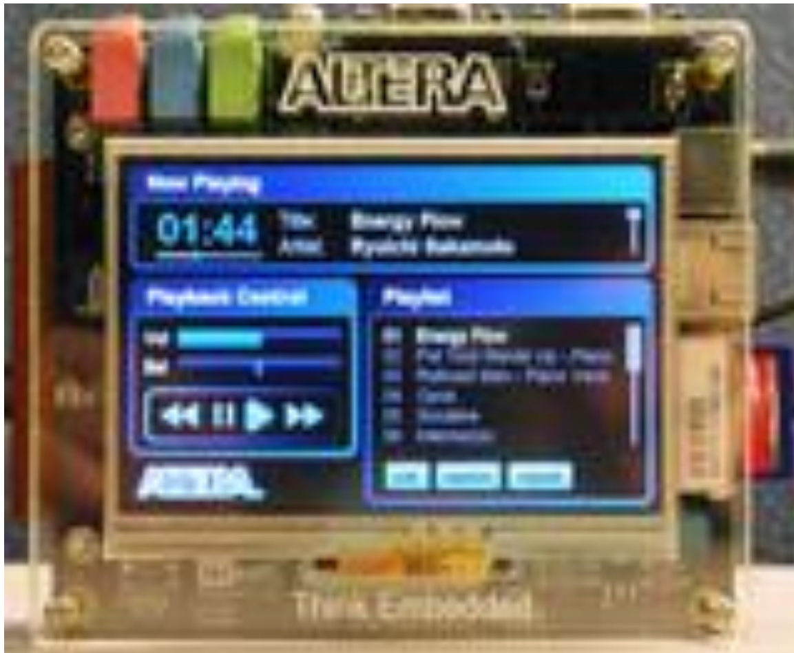
Fig. 4 Mp3 Player application on Nios II embedded evaluation kit
