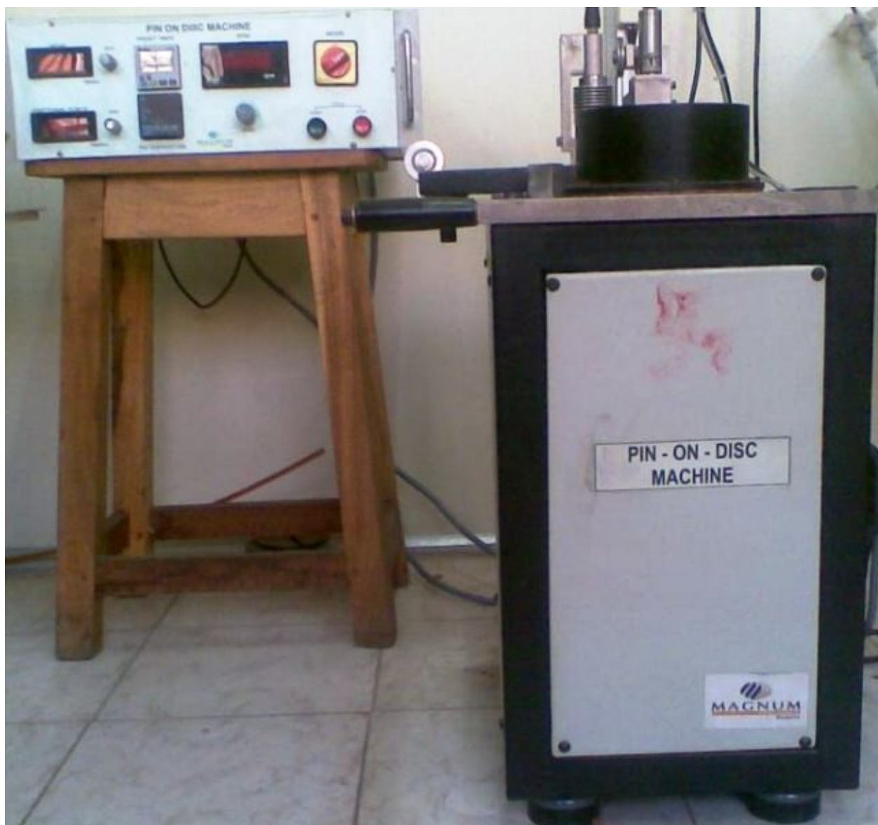
Fig 3.1: Set up to perform an Abrasive wear test on a pin on the disc
