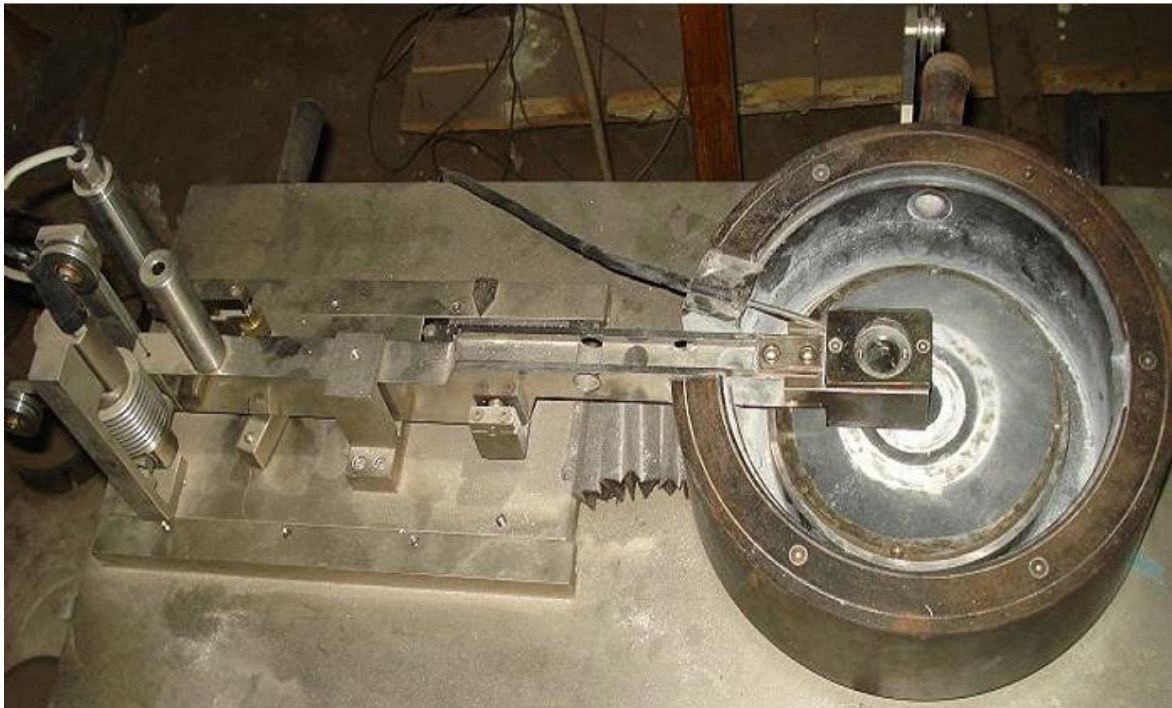
Fig3.1 DUCOM Wear and Friction Monitor used for the wear tests
