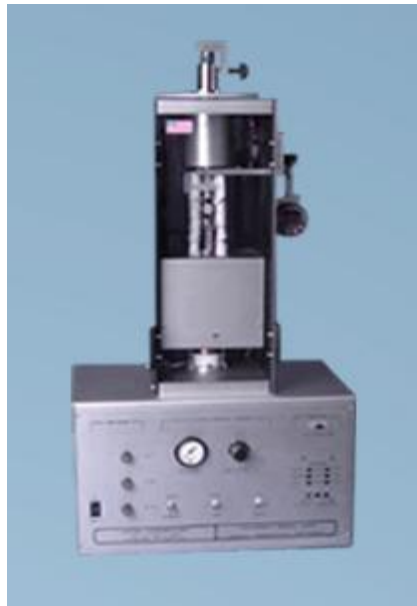
Fig. 3.2 Determination of Thermal Conductivity Using Unitherm™ Model 2022
