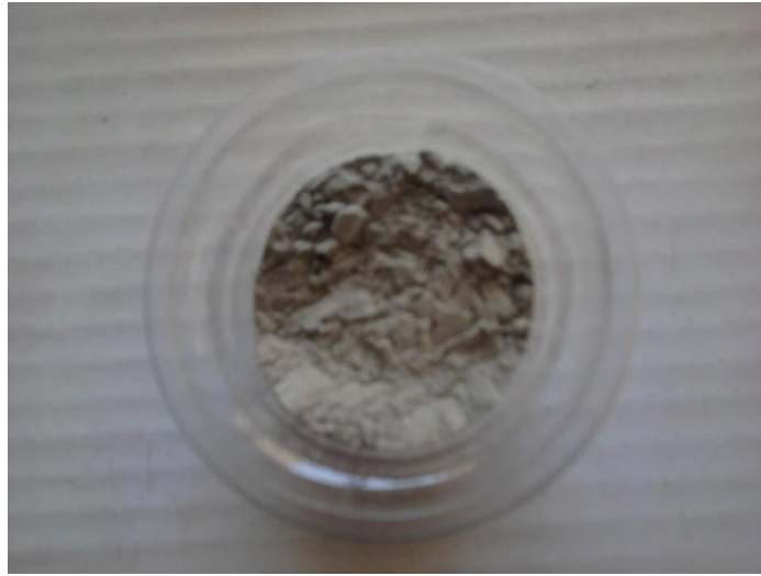
LD Slag used in the fabrication of the LDS-PEEK composite
