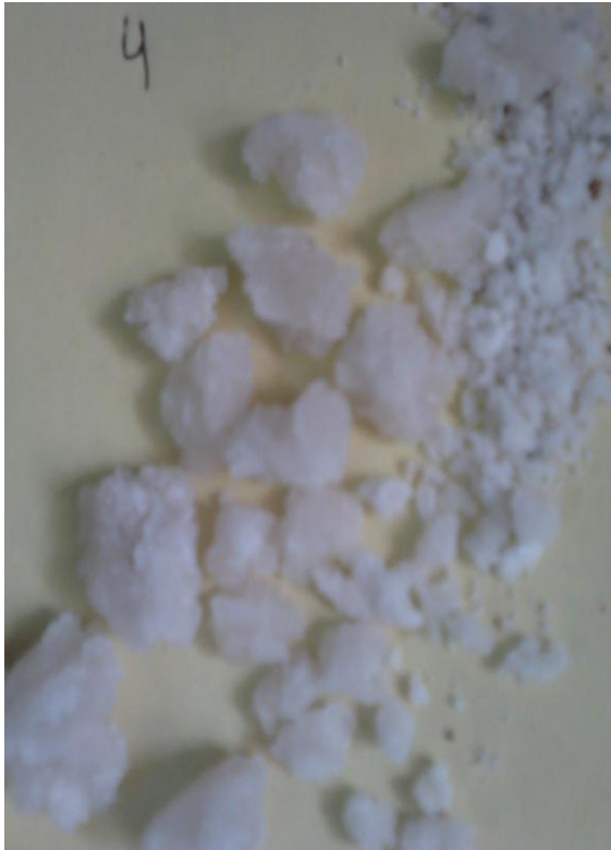
FIGURE.9: Low air velocity results in larger agglomerate particles.
