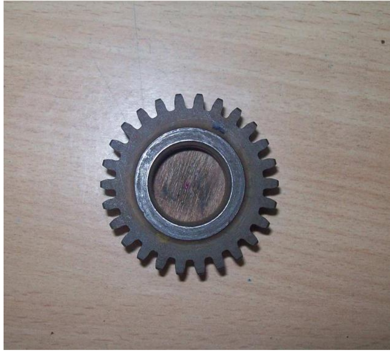
Figure 30 Pinion (spur Gear) attached to the Servo motor for rotating the Central Pinion attached to the Steering of Vehicle. Diameter of pitch circle = 45mm
