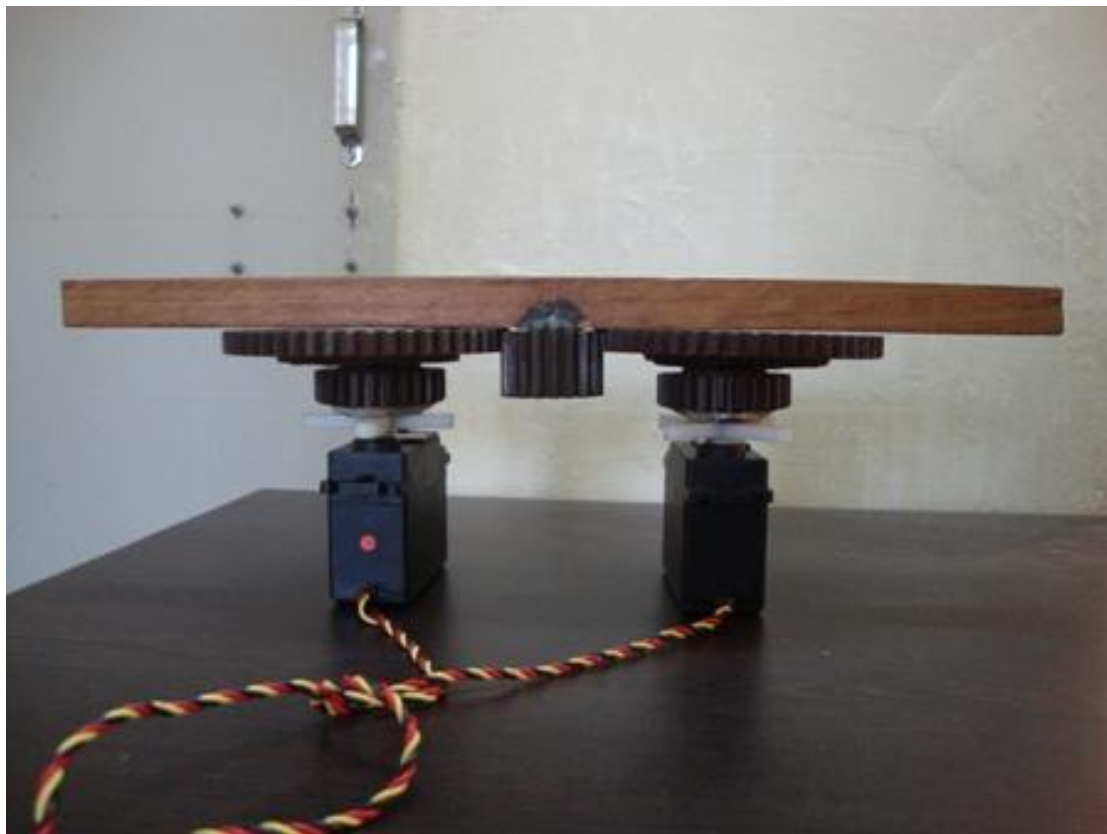
Figure 32 Shaft carrying the Central Pinion (to be attached to Steering wheel)
