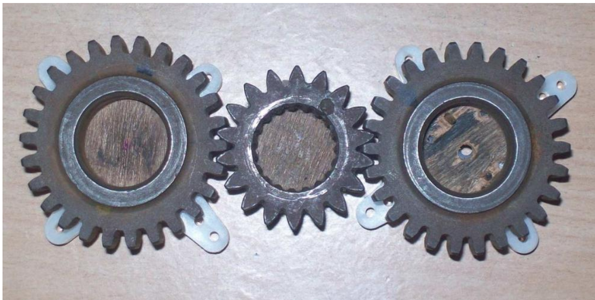
Figure 30 Pinion (spur Gear) attached to the Servo motor for rotating the Central Pinion attached to the Steering of Vehicle. Diameter of pitch circle = 45mm
