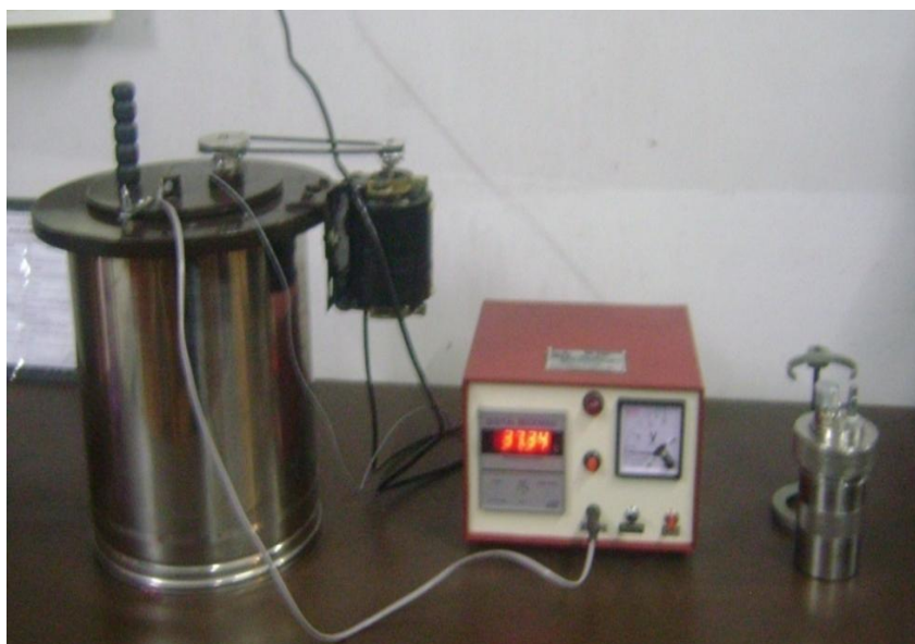
Plate 3.5 Experimental Set up of Bomb Calorimeter
