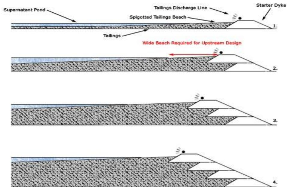
**Fig 5.3.1.1 upstream construction method**
