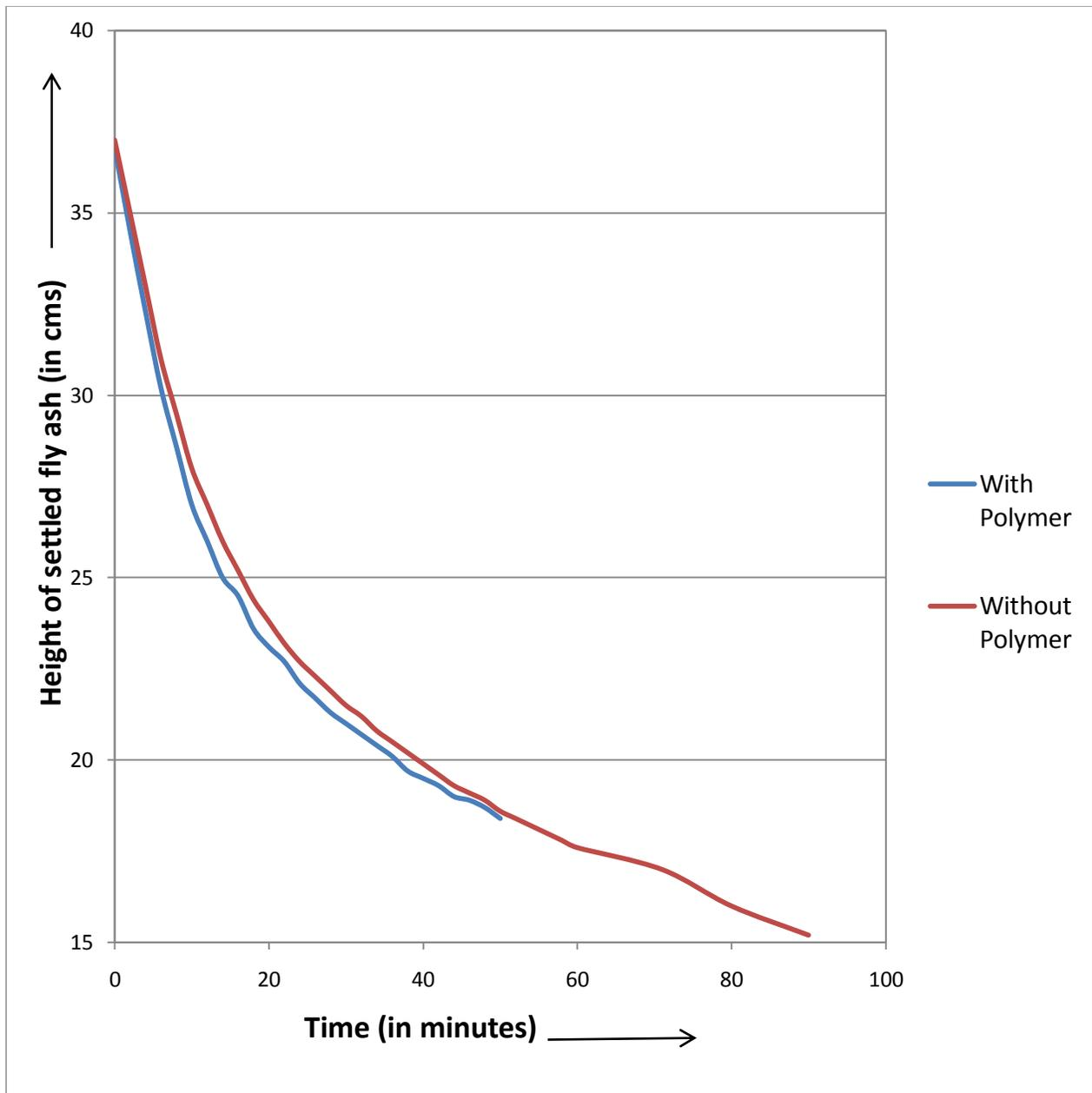
**Fig 4.4.1 Height of settled fly ash vs. time**
