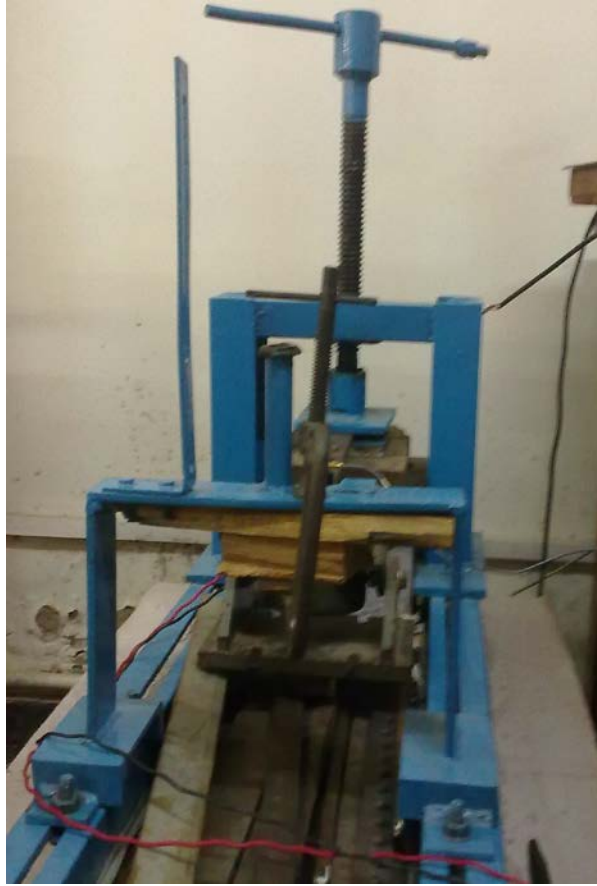
Fig. 17 Experiment set-up for fixed-fixed beam (front view)
