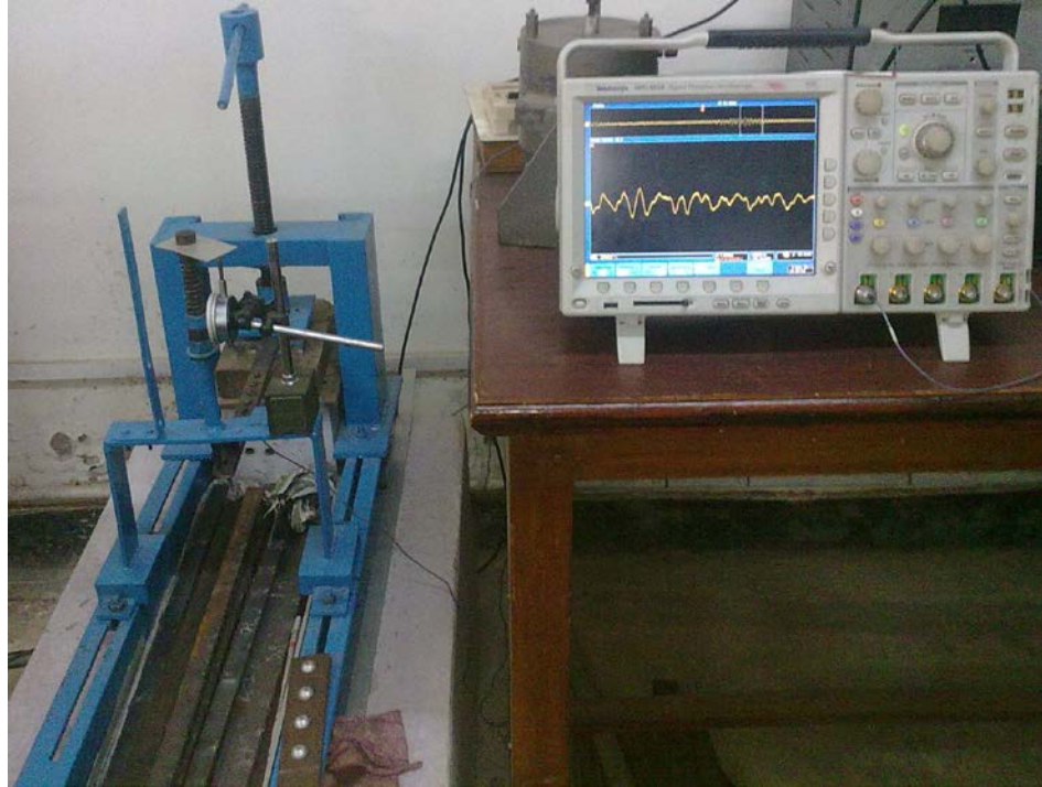
Fig. 15 Experiment set-up for cantilever beam (front view)
