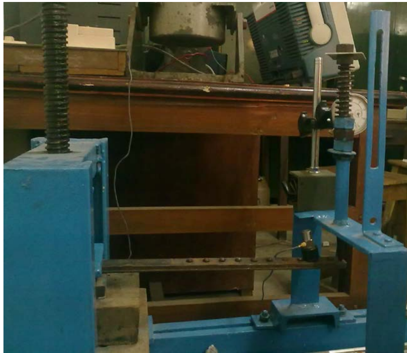
Fig. 16 Experiment set-up cantilever beam (side view)
