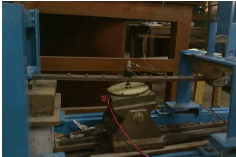
Fig. 18 Experiment set-up for fixed-fixed beam (side view)
