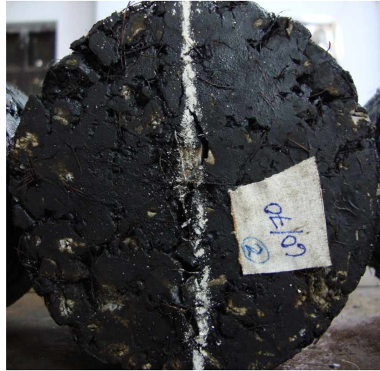
(ii) 60/70 bitumen sample
