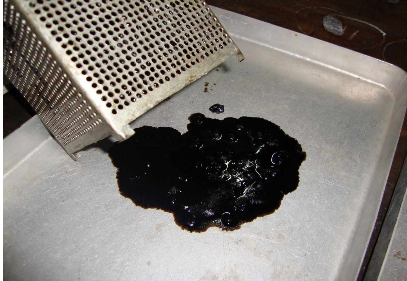
Fig. 3.4 Drainage of 80/100 bitumen sample
