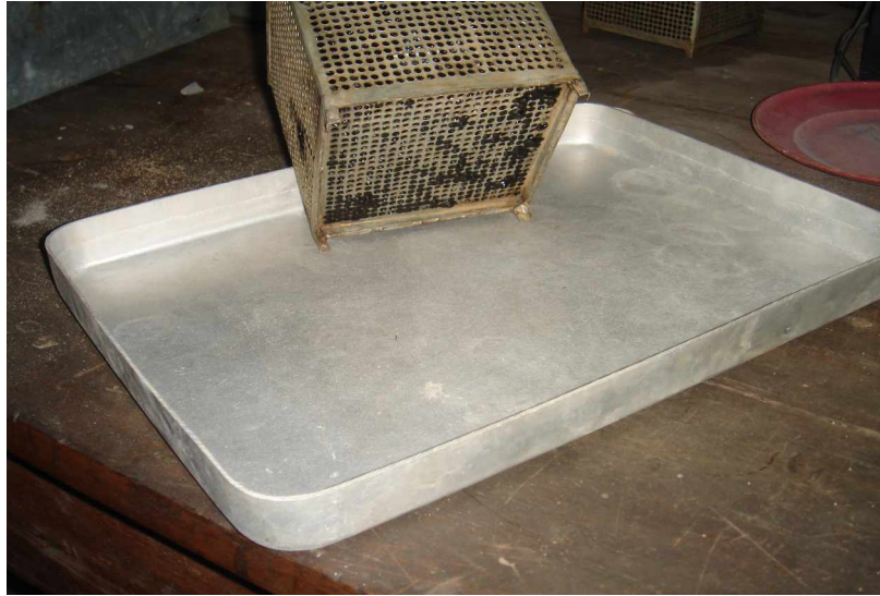
Fig. 3.6 Drainage of CRMB 60 binder sample
