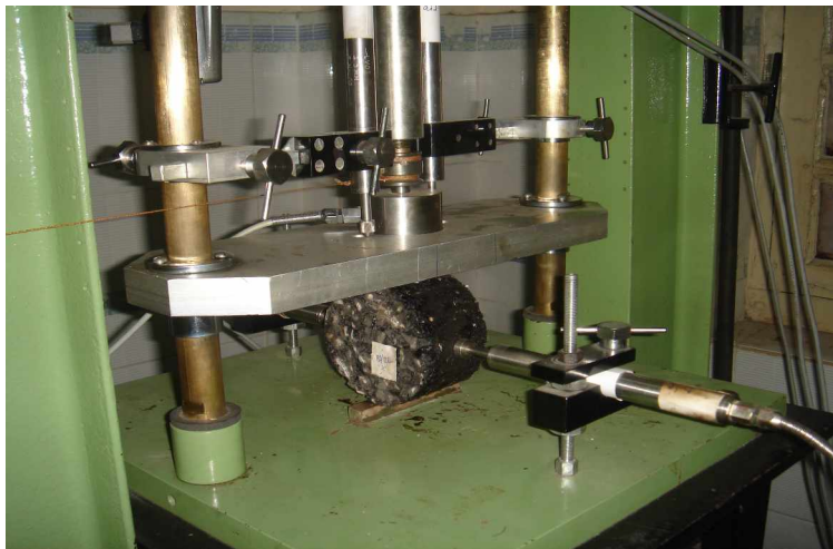
Fig. 3.14 Close view of a loaded sample in repeated load indirect tensile test
