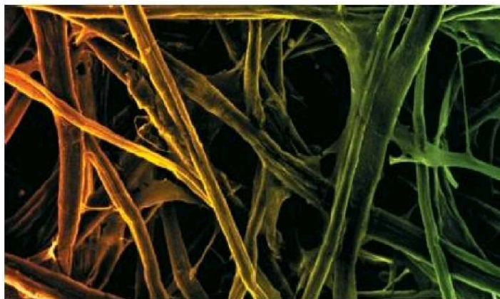
Fig.2.5 Appearance of cellulose fiber under scanning electron microscope
