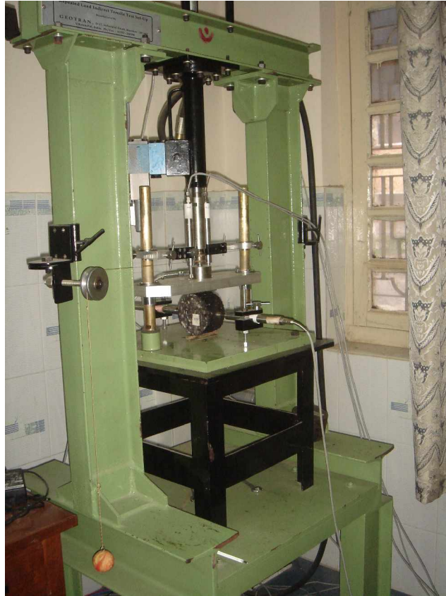
Fig. 3.13 A photograph of repeated load indirect tensile test setup
