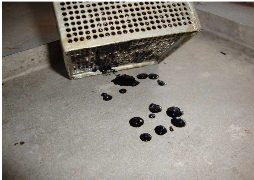
Fig. 3.5 Drainage of 60/70 bitumen sample
