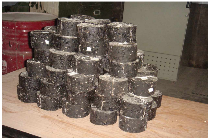
Fig. 3.16 Some of the samples tested in repeated load indirect tensile test
