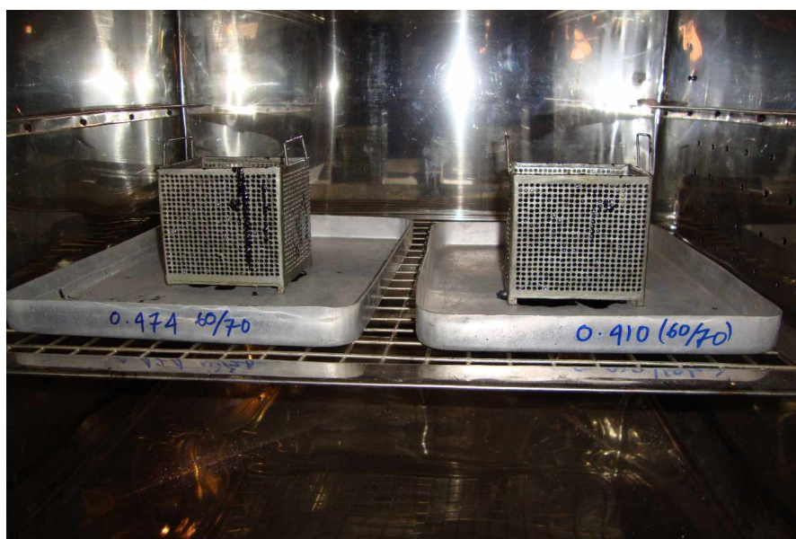
Fig. 3.3 Drainage baskets kept in oven at 150°C
