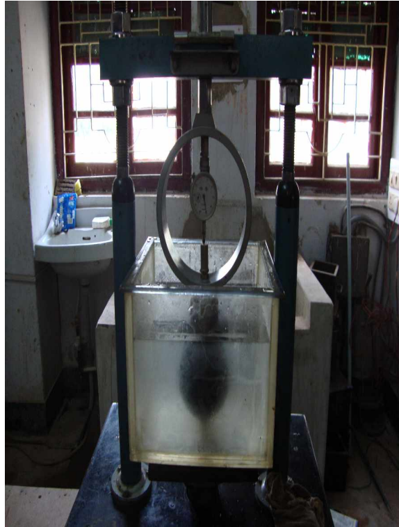
Fig. 3.7 Static indirect tensile test in progress
