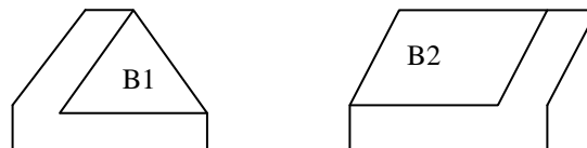
Figure 4.3(a) Generating the configuration space obstacle B1A
