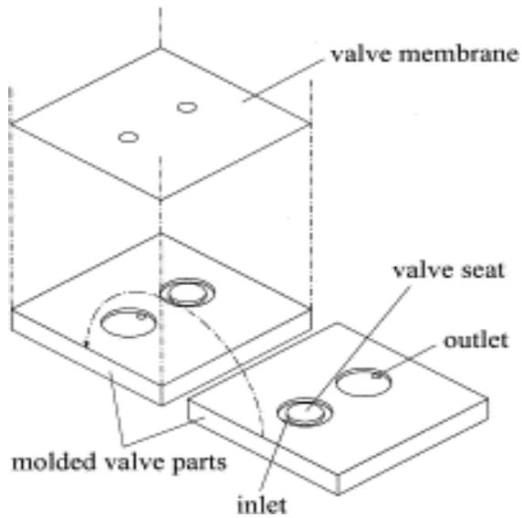
Sandwich construction of two molded plastic valve parts and a thin punched membrane in between.
