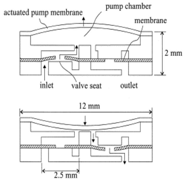
Cross-section of the pump showing the directions of flow for different actuating phases.
