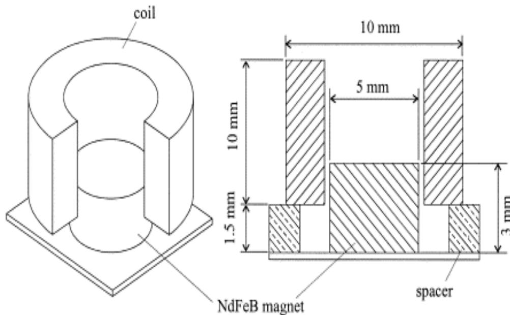
Construction of the electromagnetic actuator. Dimensions are in millimeter.
