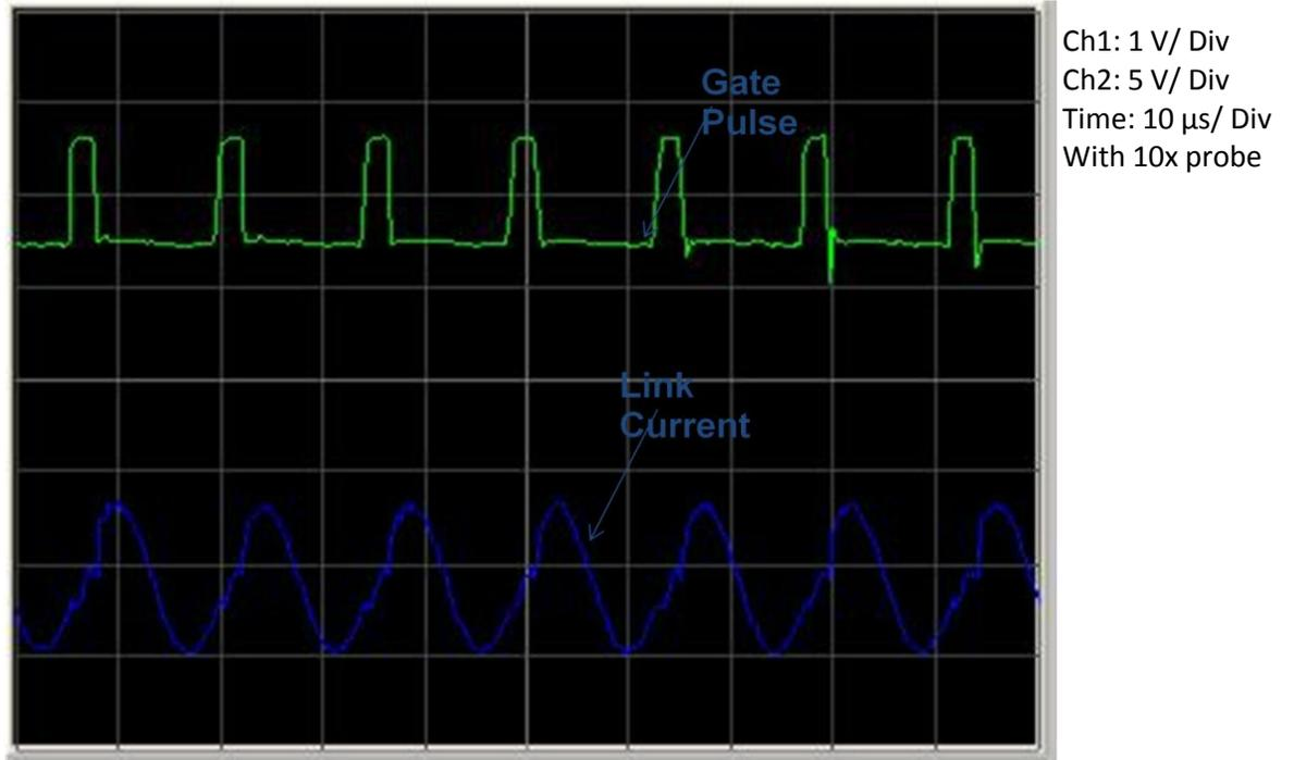
Figure 5. 5: Gate Pulse and Link Current
