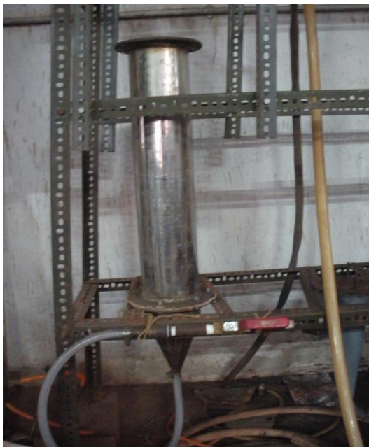
Figure 2: Photograph of designed fluidized bed reactor
