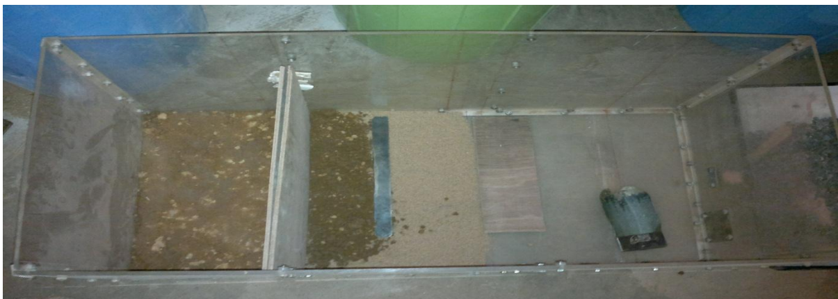
Fig.4.23 Making Of The Starter Dyke With Clay
