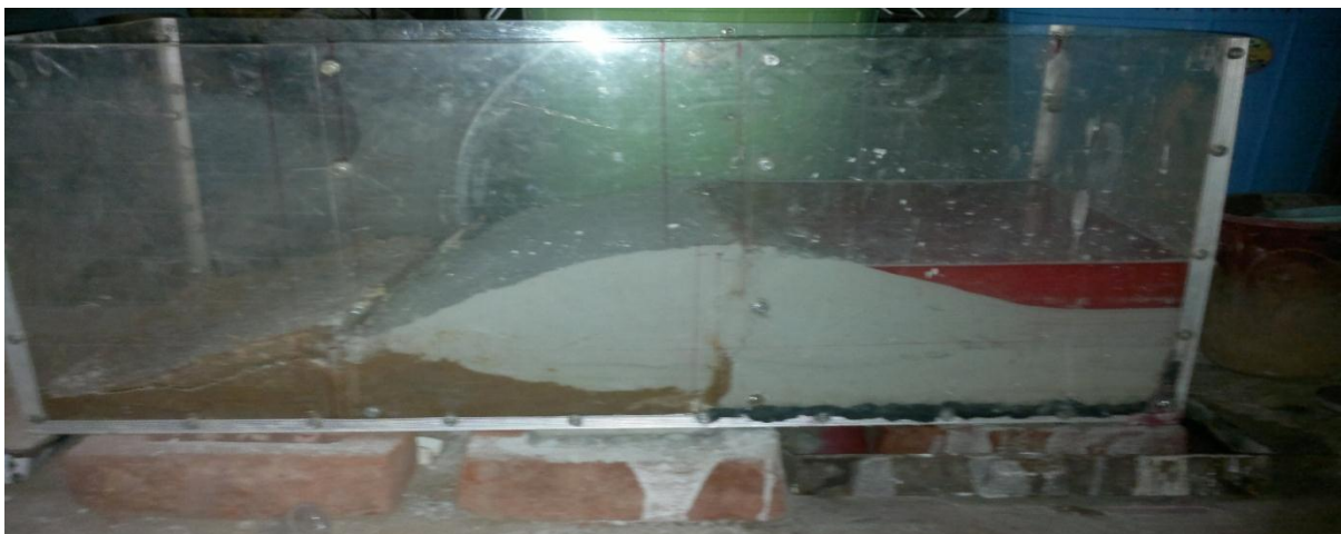
Fig.4.29 Leakage Of Slurry
