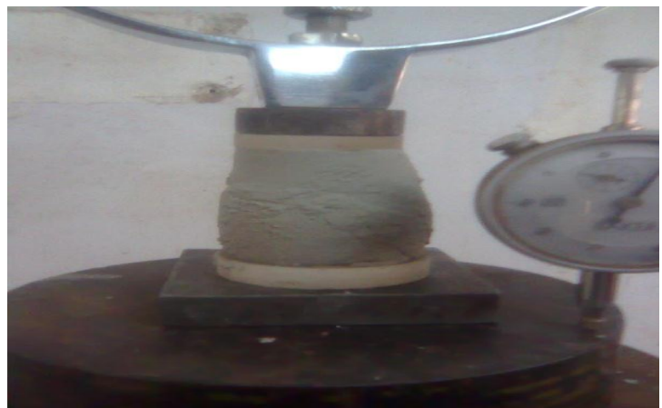
Fig. 4.7 Failure Of Fly Ash Specimen in unconsolidated compressive test
