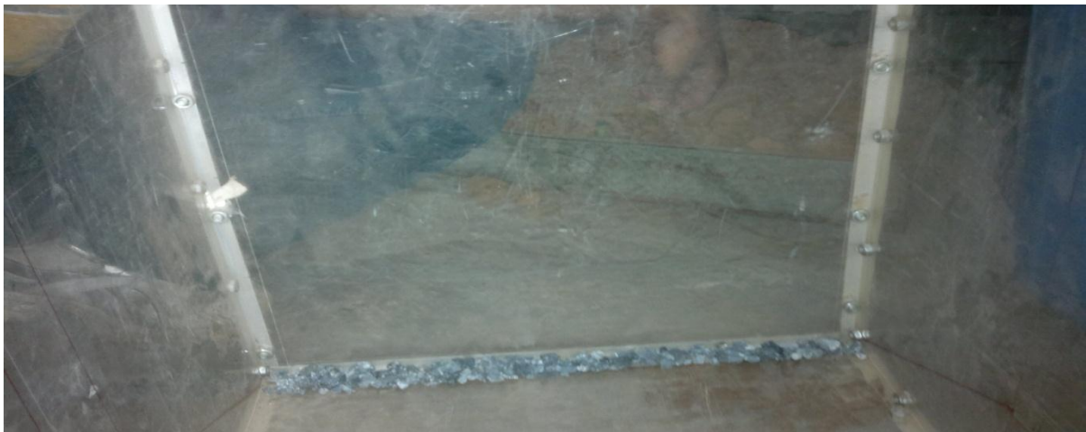
Fig.4.21 Placing Of Toe Filter In The Model
