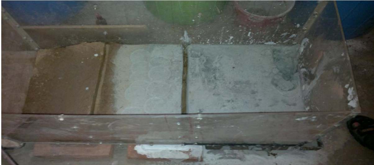
Fig.4.26 Compaction Of Slurry Up To Starter Dyke
