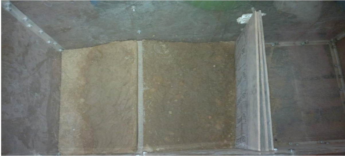
Fig.4.24 Placing Of Vertical Drain Filter In The Model
