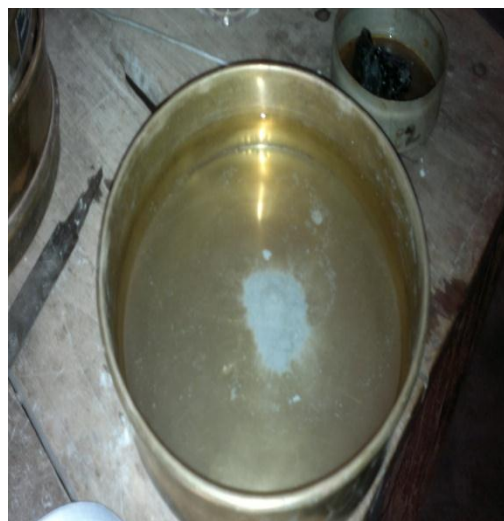
Fig. 4.9 Crumb Test Of Fly Ash
