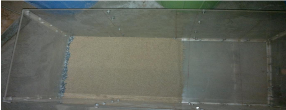
Fig.4.22 Placing Of Horizontal Filter In The Model
