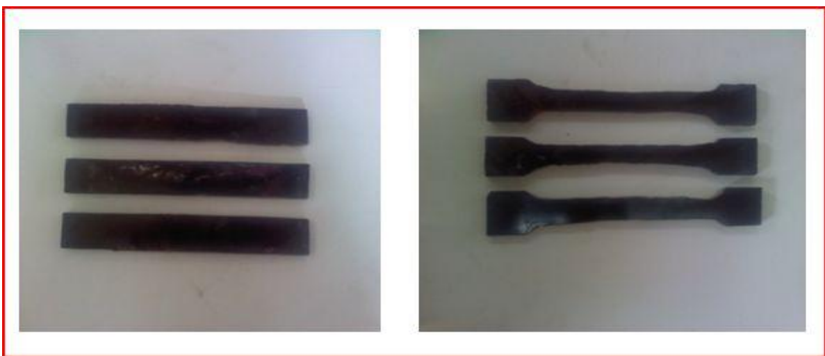
Figure 3.7 Specimen for Flexural test
