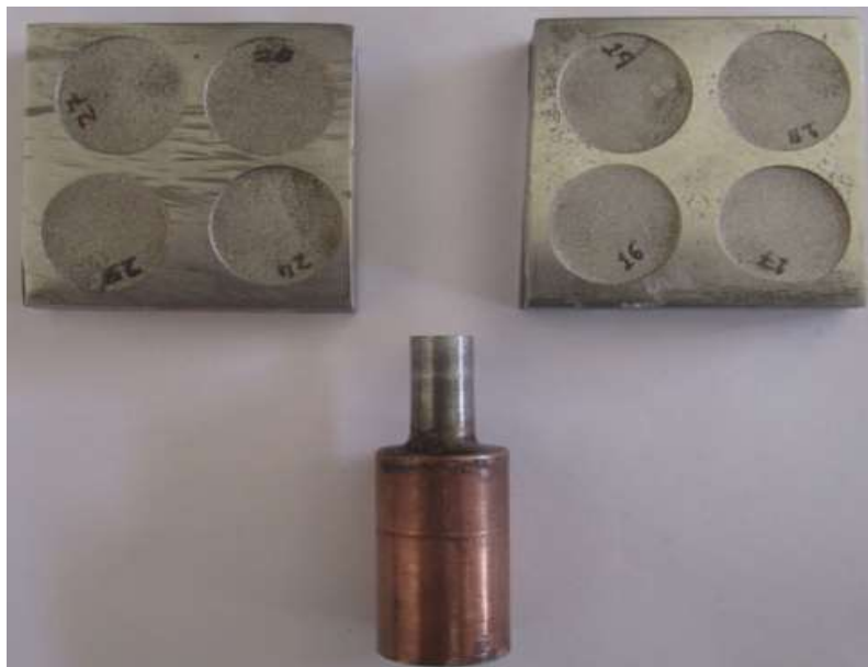
Fig. 3.3 Machined workpiece and Tool
