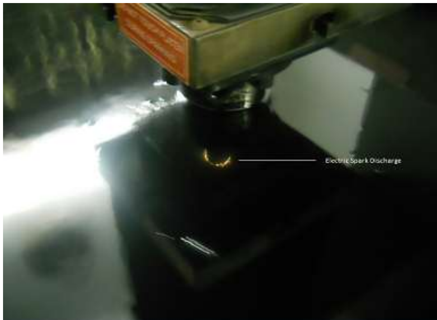
Fig. 3.4 Spark produced during machining
