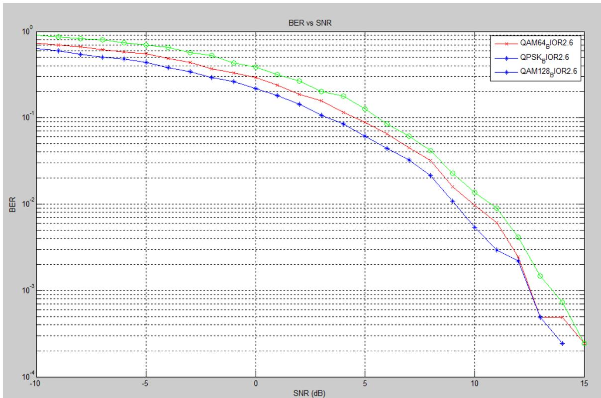
Figure 16: BER vs. SNR for different types of constellation Encoding in AWGN channel for haar wavelet
