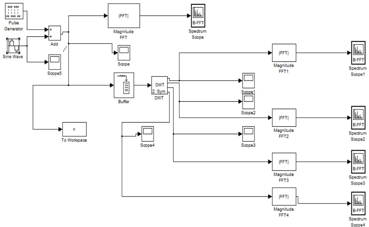
Figure 12: Model based design for Wavelet packet decomposition in Simulink
