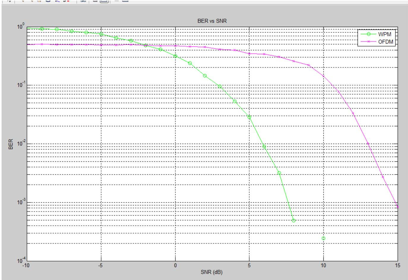
Figure 20: BER vs. SNR plot for comparison of performance of OFDM and WPM
