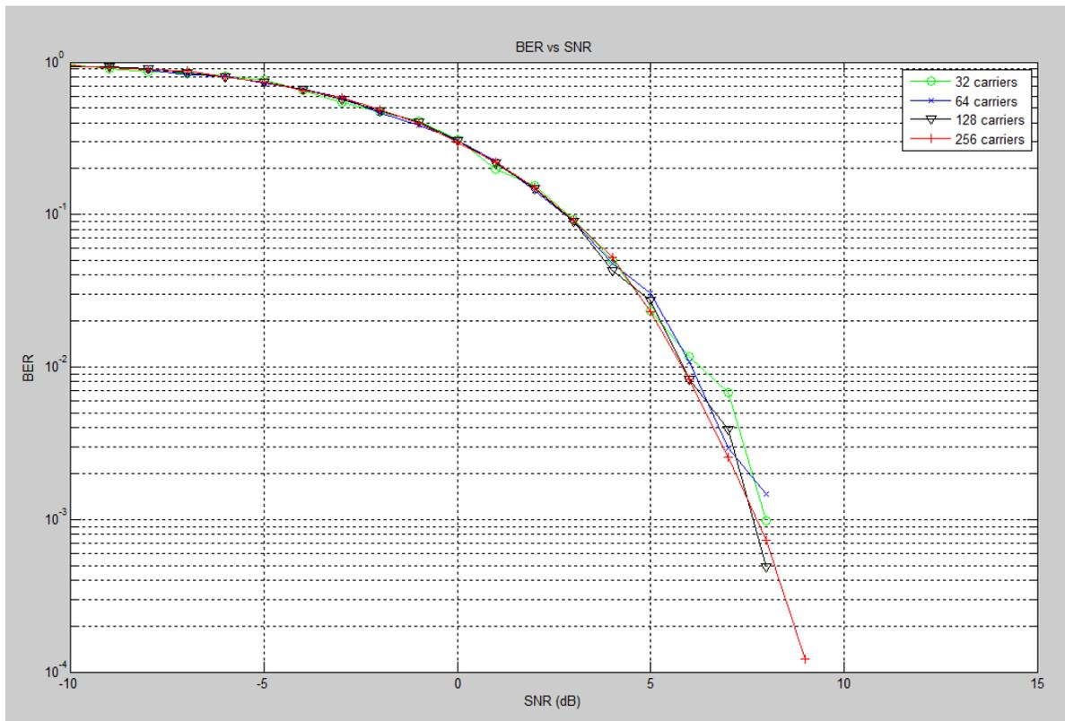
Figure 17: BER vs. SNR for different number of carriers for haar wavelet in AWGN channel
