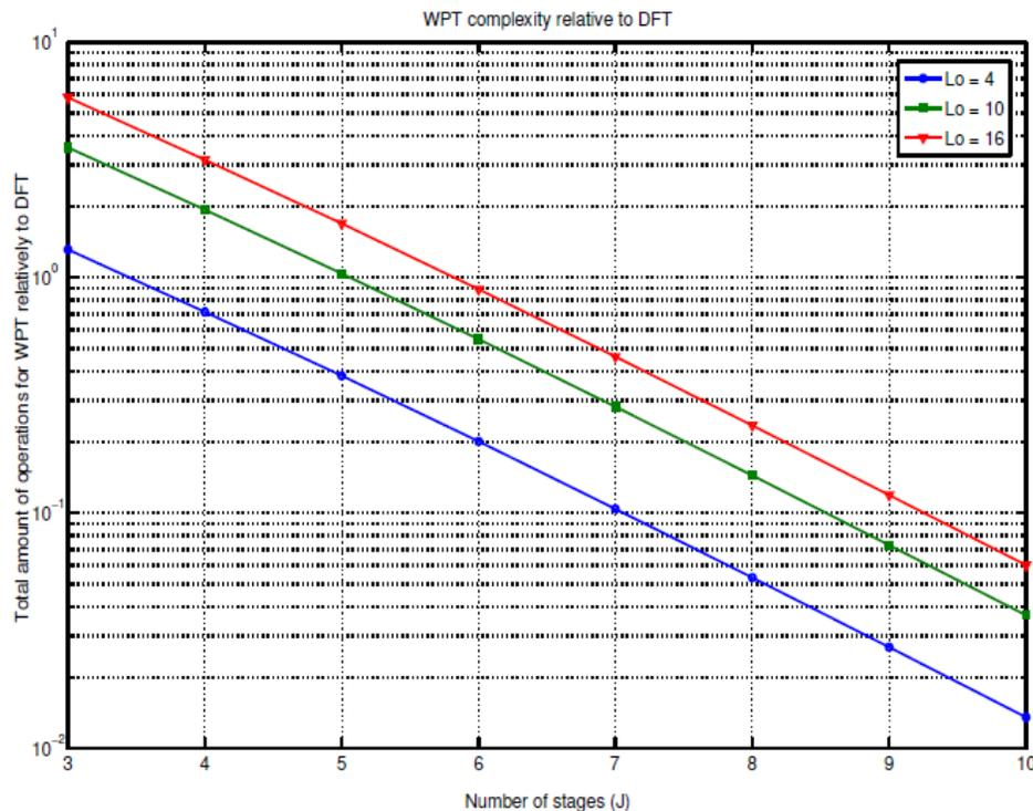
Figure 22: WPT complexity relative to that of the DFT as a function of the transform size [2]
