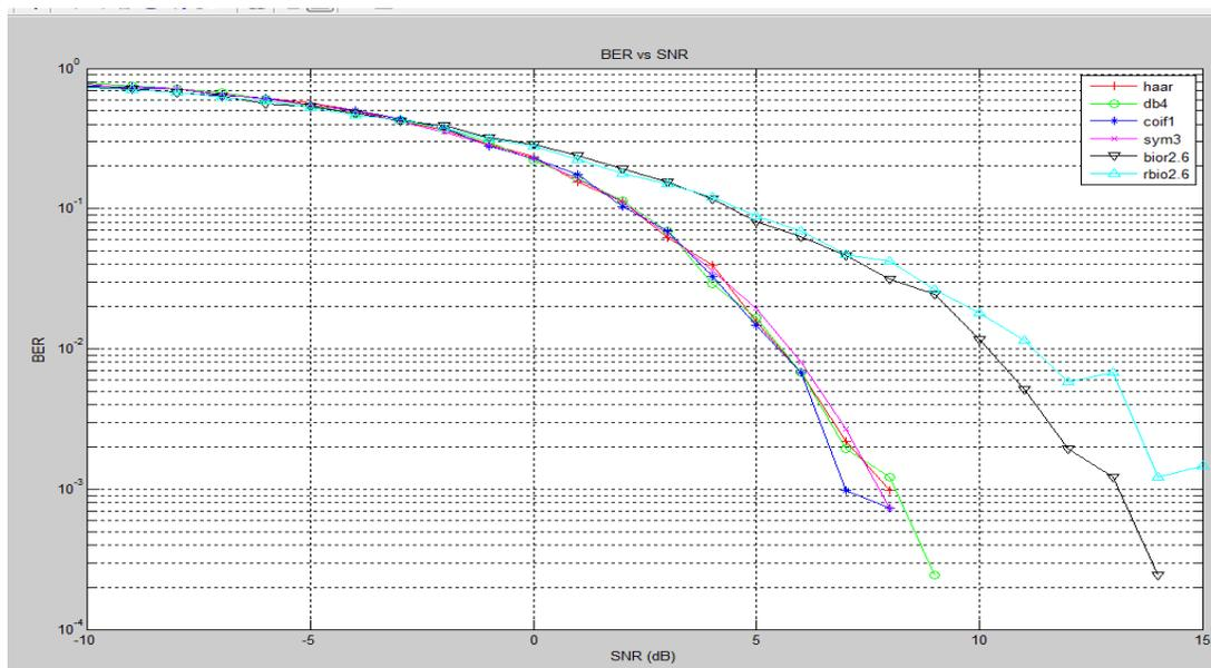
Figure 19: BER vs. SNR plot of different wavelet families for 64-QAM encoder WPM
