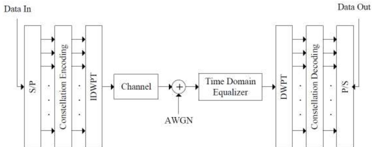
Figure 9: Block diagram of WPM (System Model) [2]
