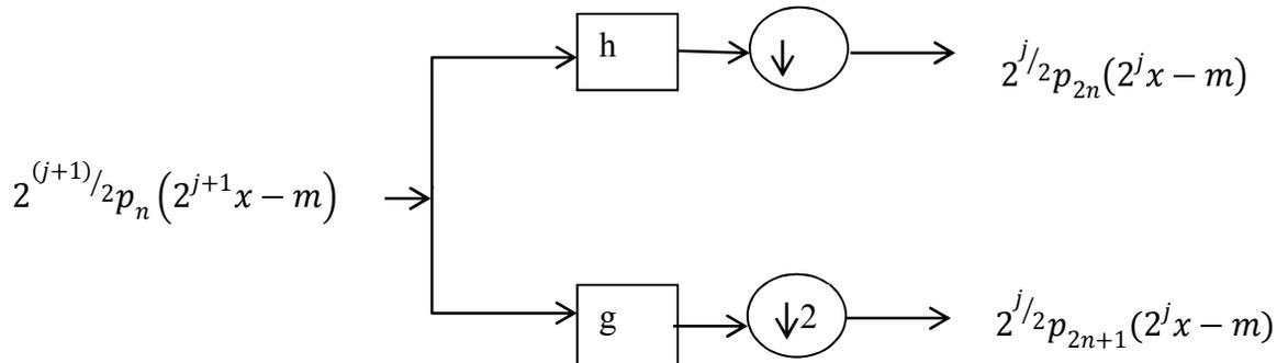
Figure 8: Wavelet packet decomposition by two-channel filter bank.[2]
