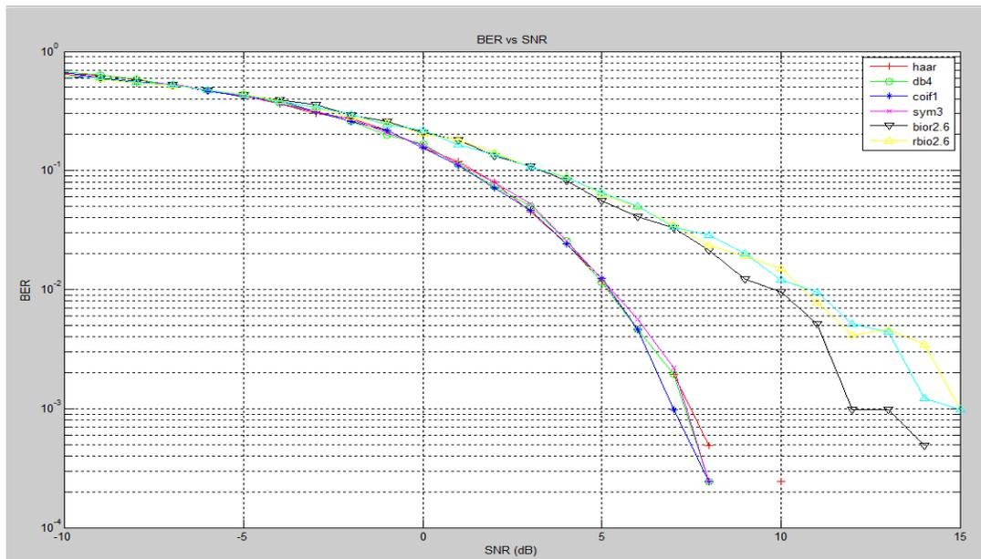
Figure 18: BER vs. SNR plot of different wavelet families for QPSK encoder WPM
