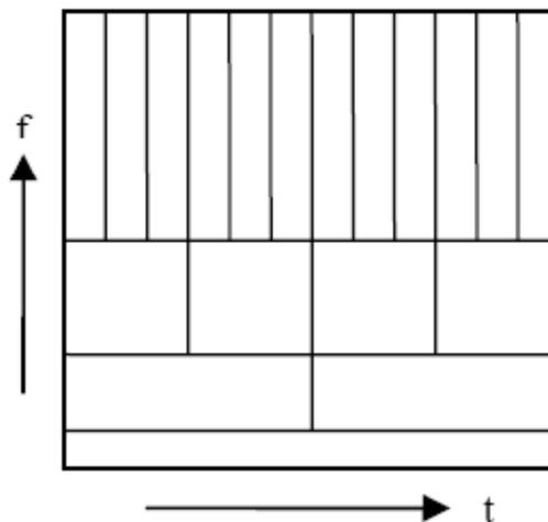
Figure 6 – Resolution of time and frequency in Wavelet Transform [9]
