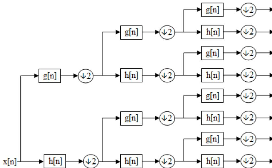
Figure 7: Wavelet Packets of 3 levels of decomposition of signal  $x[n]$  [3]
