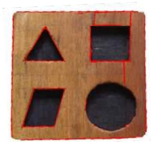
Fig 4.13 Detected edge on original image
