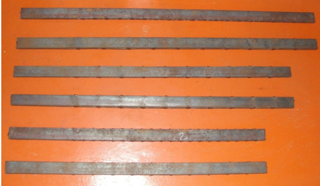
Fig-2 (Top view of mild steel specimen)
