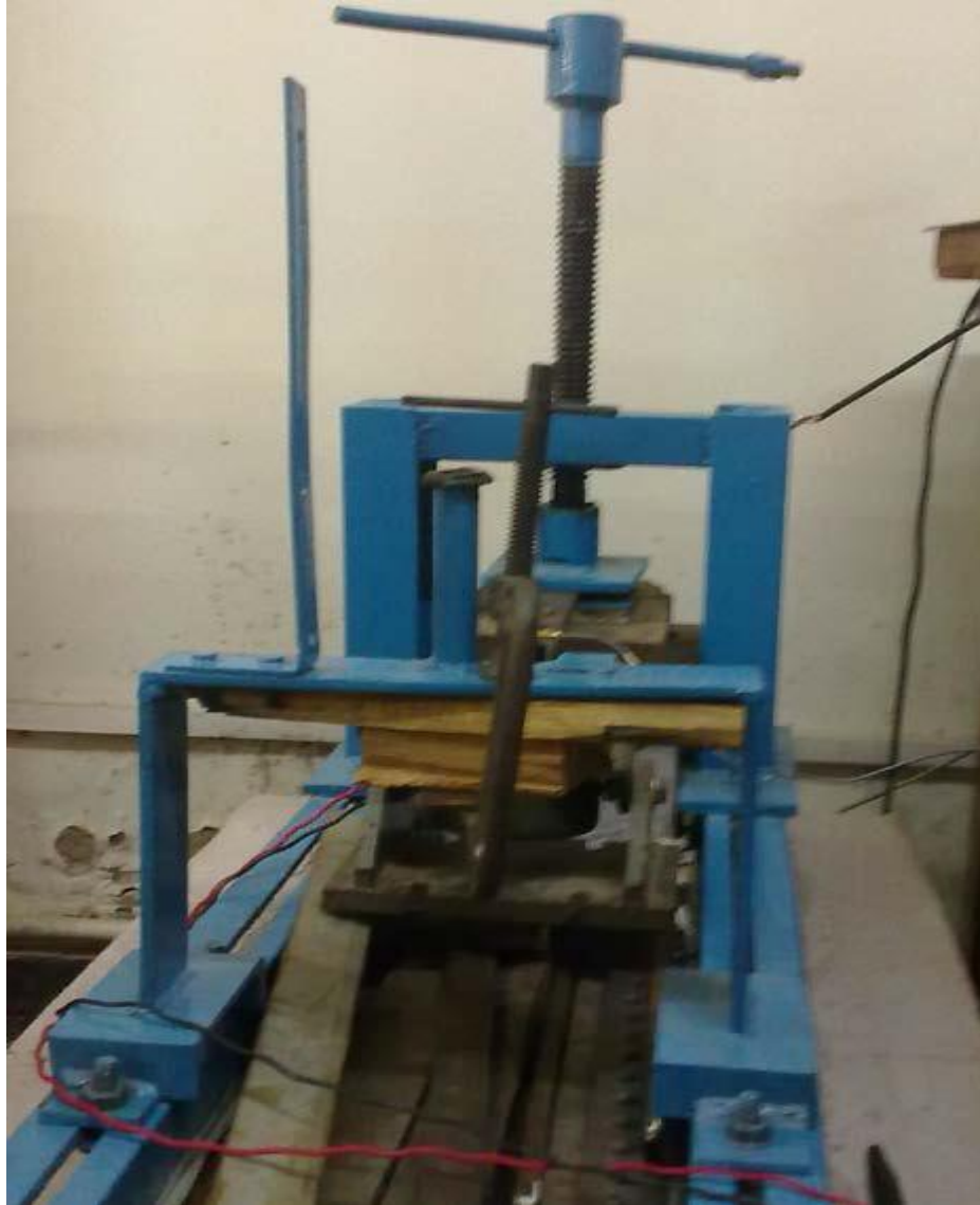
Fig-4 (Experimental set up fixed fixed beam)
