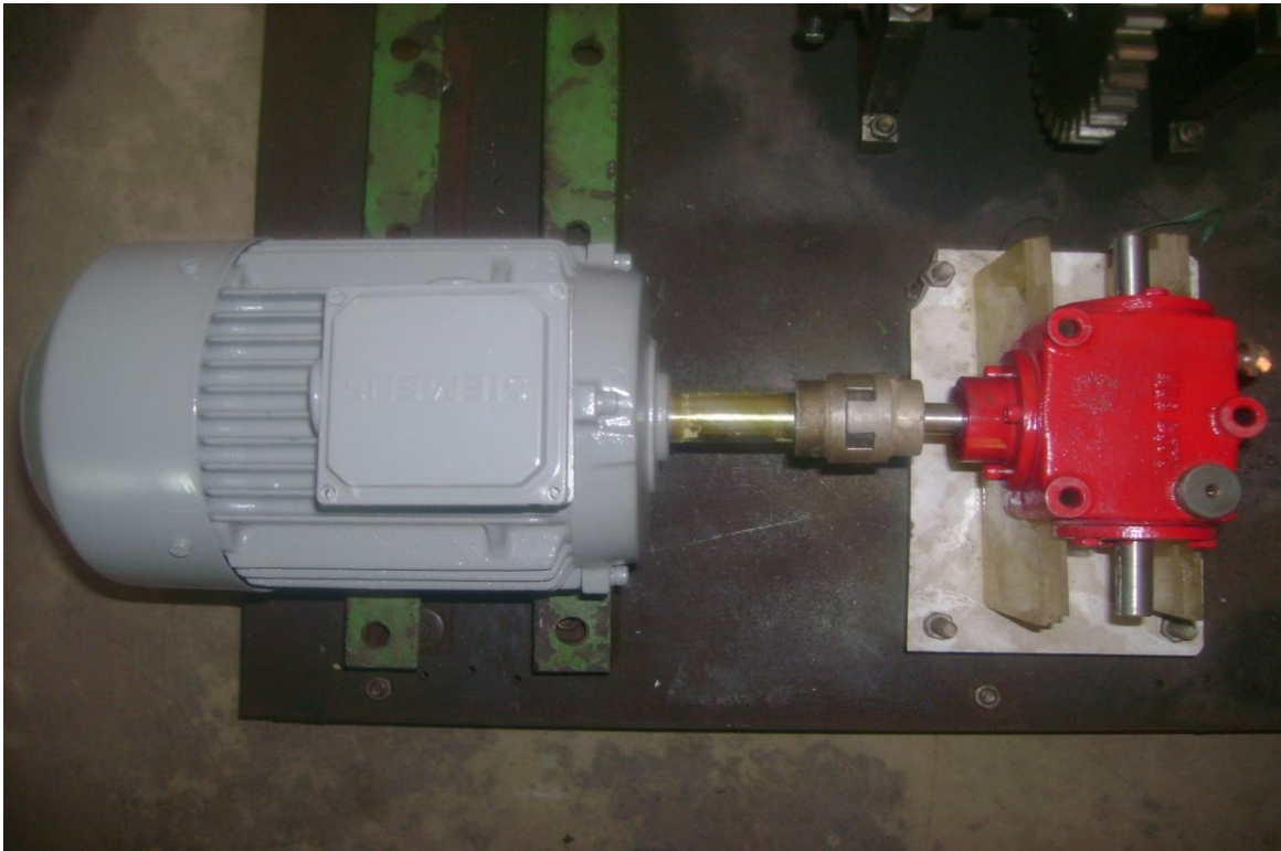
Fig: 16. Motor coupled with the gearbox.
