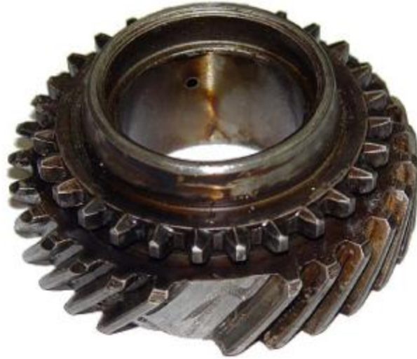
Fig: 4. Gear with two broken teeth.
