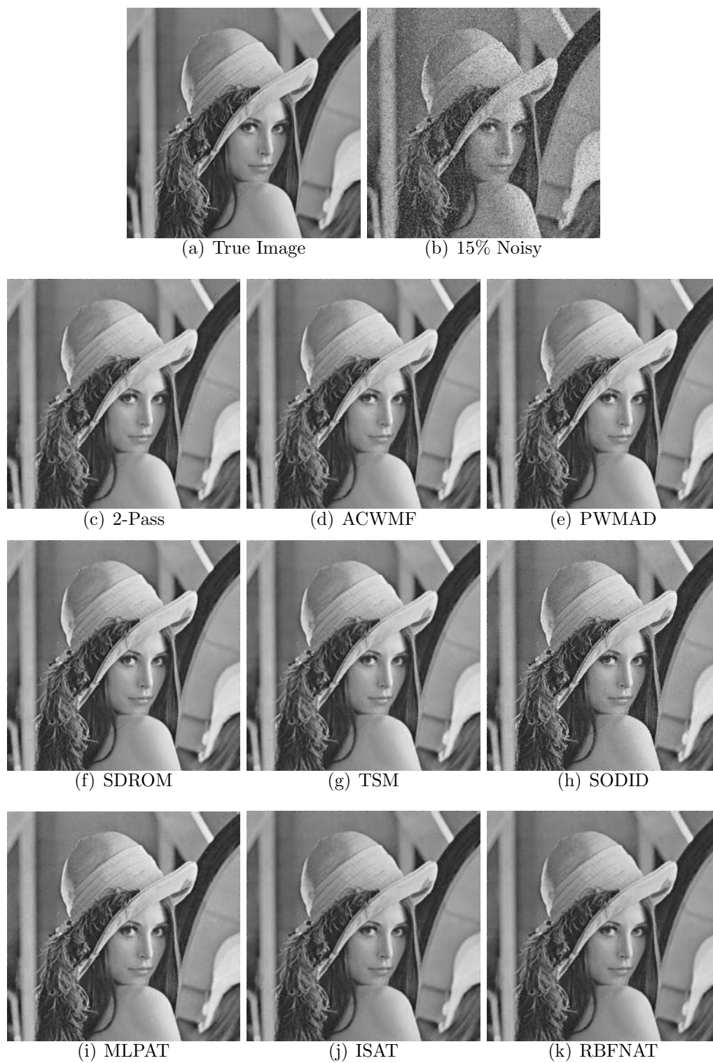
Figure 2.15: Impulsive Noise filtering of Lena image corrupted with 15% of RVIN by different adaptive threshold schemes
