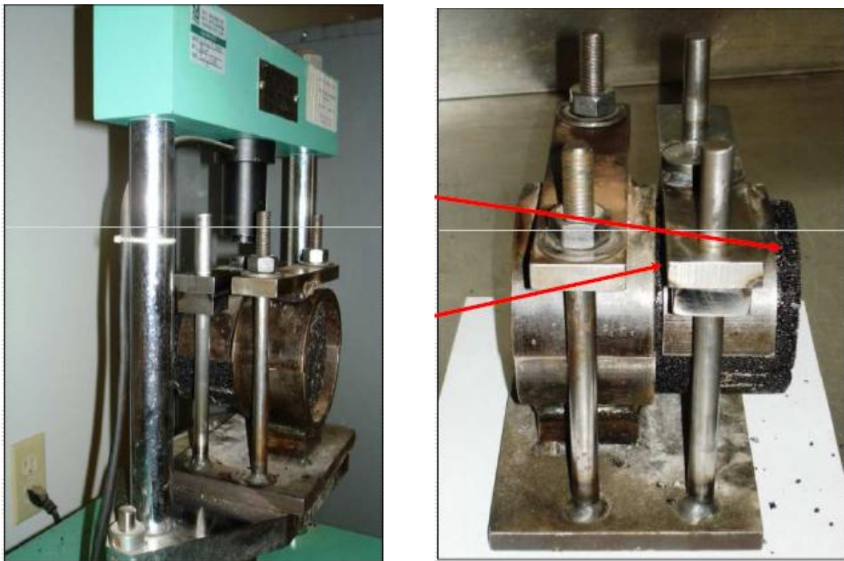
Figure 2.8: Shear-Testing device developed at McAsphalt Lab (Tony Kucharek et al.)
