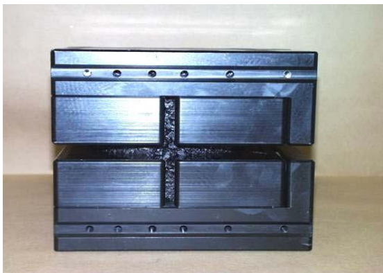
Figure 2.3.1: Shear Box with Prepared Specimen (Mohammad et al., 2002)
