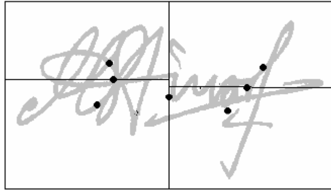
Fig 2.5: Feature points extraction based on vertical splitting
