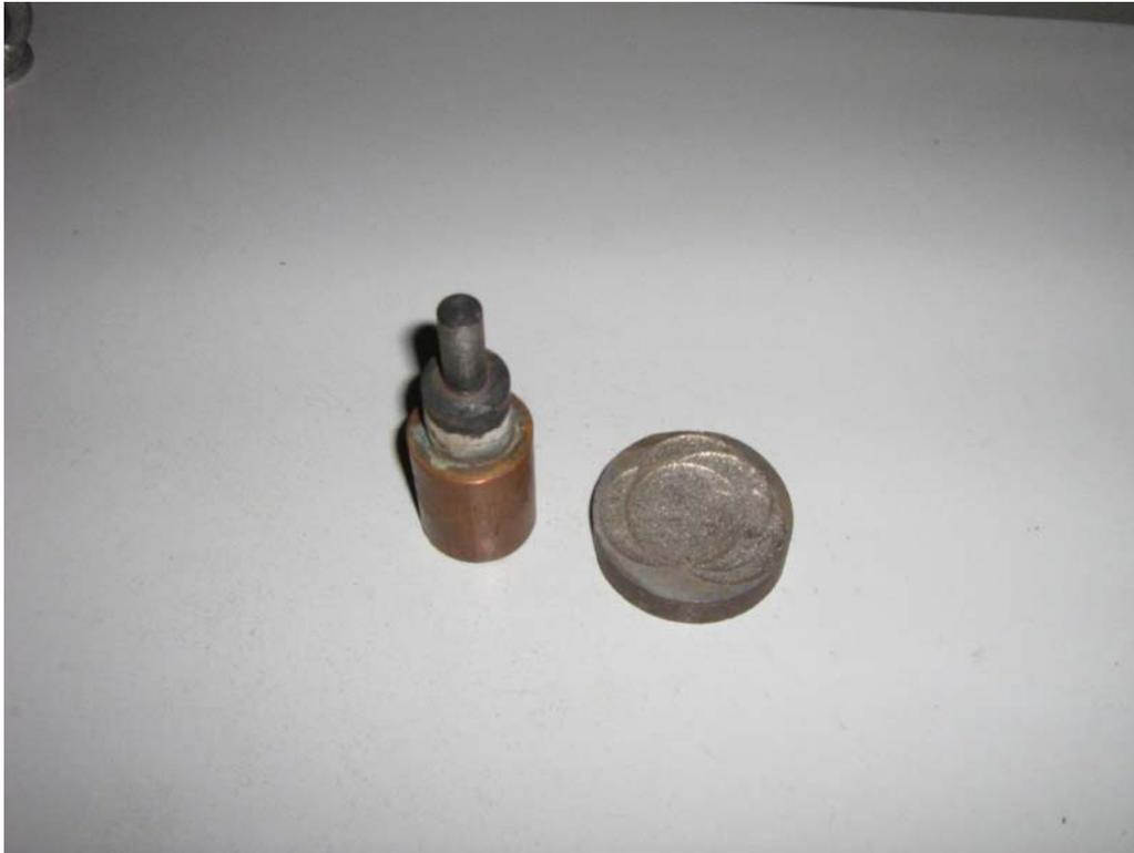
**Fig.4.5** shows the electrode and work piece after the machining operation.
