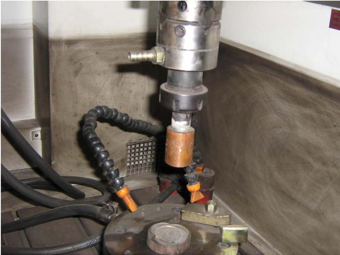
**Fig. 4.2** Electrode and work piece material used in the experiment
