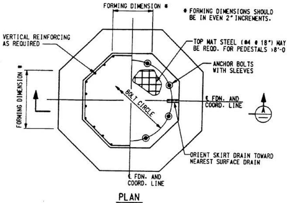
**Fig 1:** Plan of pedestal and foundation (ref. STE03350 - Vertical Vessel Foundation Design Guide)
