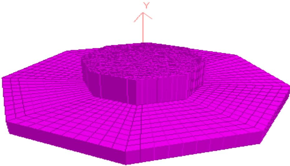
**Fig.3** STAAD model of the pedestal and footing
