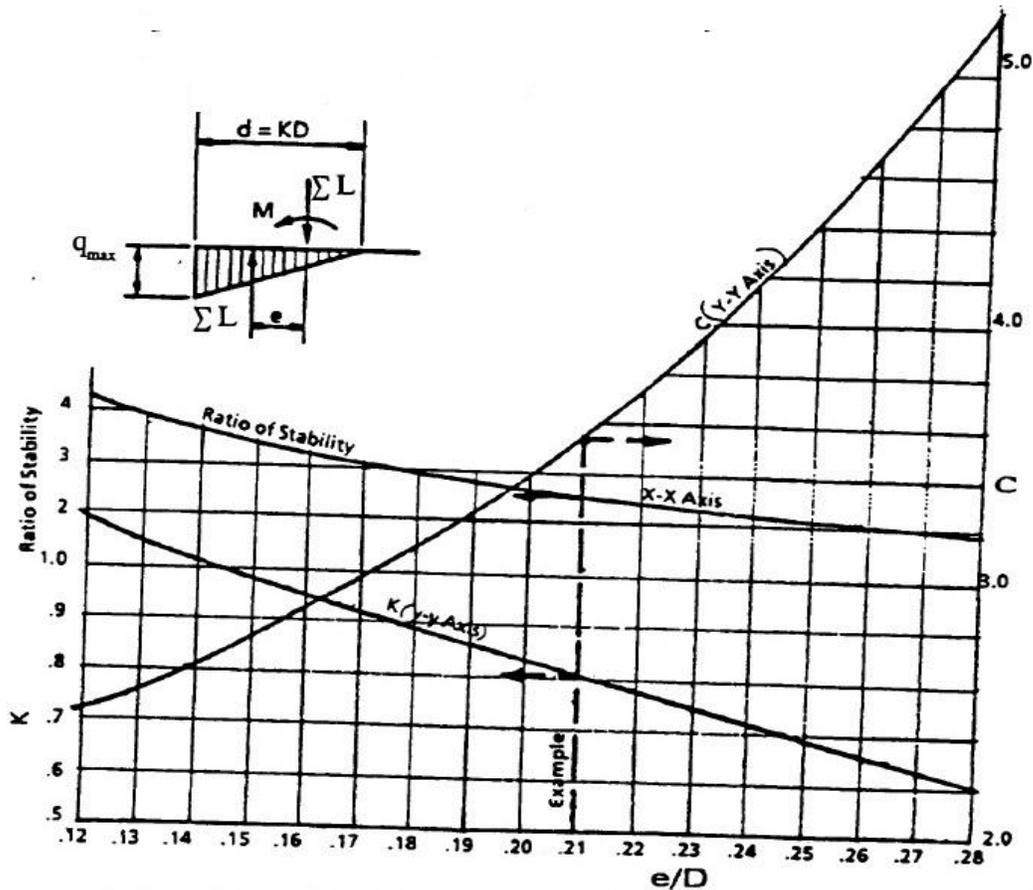
Fig 2. Graph for calculation of  $L_{diag}$  of octagonal footing. ref. STE03350 - Vertical Vessel Foundation Design Guide
