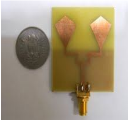
THE FABRICATED 1×2 DIAMOND SHAPED MICROSTRIP PATCH ARRAY
