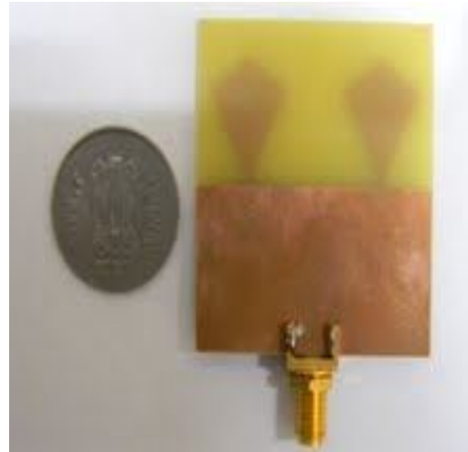
THE FABRICATED 1×2 DIAMOND SHAPED MICROSTRIP PATCH ARRAY
