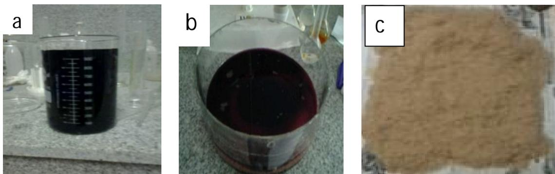
Fig 3.4(a) 0.01N  $\text{KMnO}_4$ , (b) sand soaked in 0.01N  $\text{KMnO}_4$ , (c) oven dry manganese modified sand
