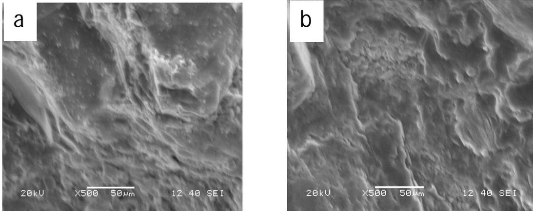
Fig 5.1(a) SEM image of uncoated sand, (b) SEM image of Manganese modified sand with 500 x magnifications
