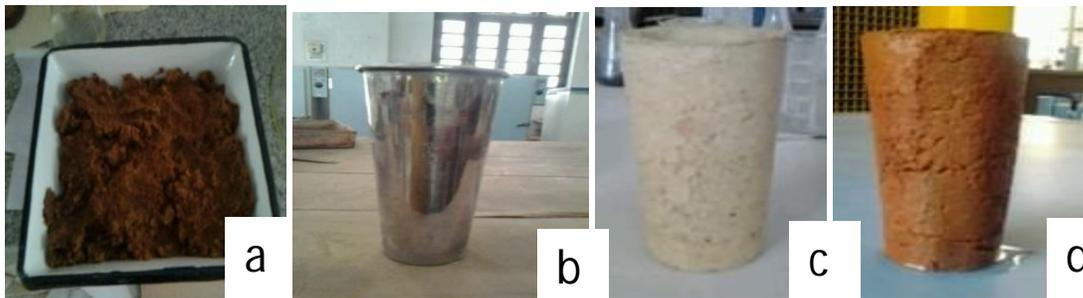
Fig 3.9(a) mixture of clay rice husk and admixtures, (b) cylindrical Mould, (c) filter after oven drying, (d) Ceramic filter after sintering at 866 degree Celsius
