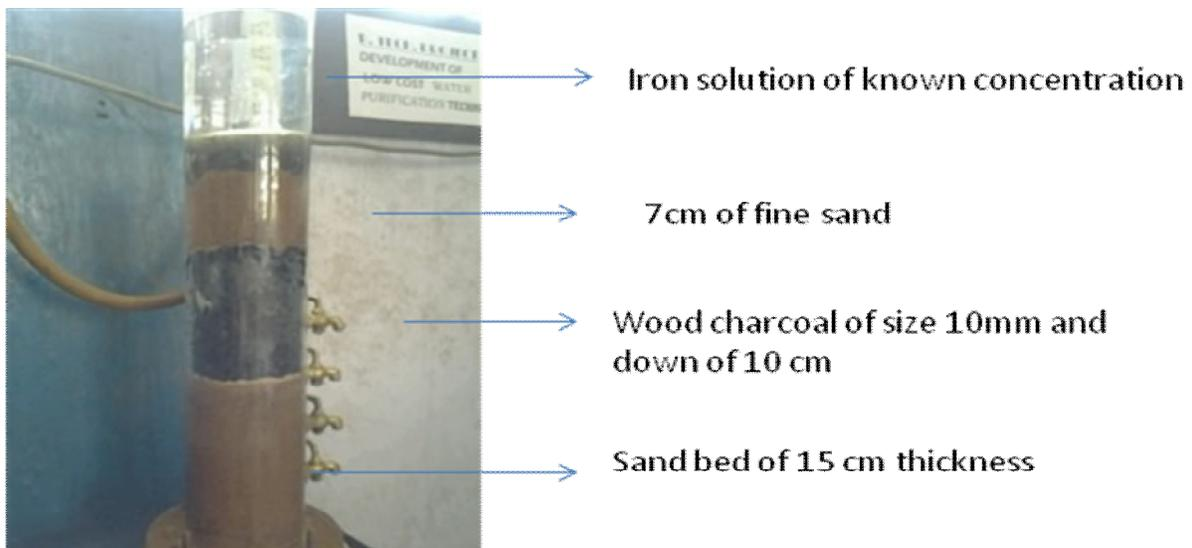
Fig 4.3 Filtration using wood charcoal as adsorption media
