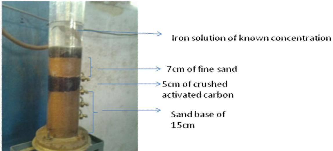
Fig 4.2 Filtration using Activated carbon as adsorption media
