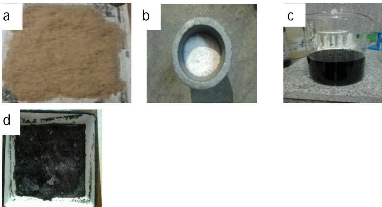
Fig 3.6 (a) Rice husk ash prepared after controlled heating at 500 degrees, (b) RHA soaked with 0.01N HCl, (c) Al(OH)<sub>3</sub> coated RHA
