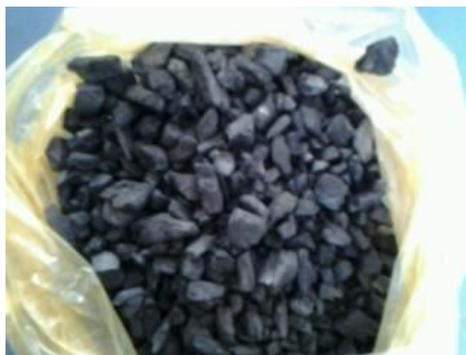
Fig 3.3 Crushed Wood charcoal of size 10mm and down
