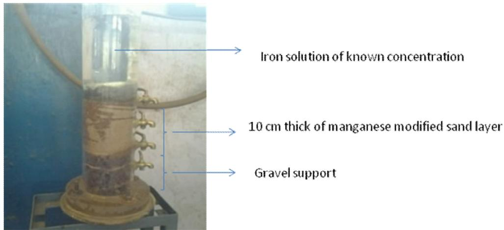
Fig 4.5 Filtration by manganese modified sand
