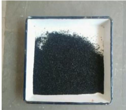
Fig. 3.2 Activated Carbon of Aqua Guard crushed into size of 2mm and down
