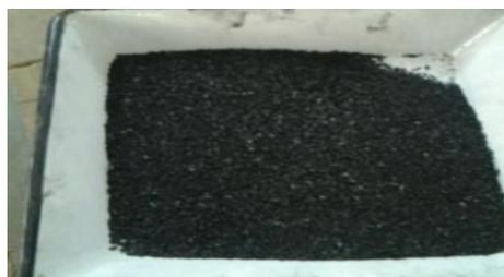
Fig 3.5 Crushed anthracite of size 625 micron and down
