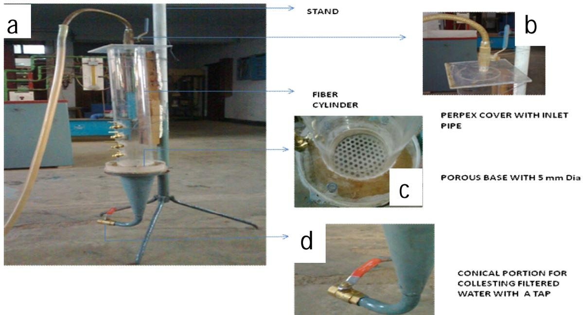
Fig. 3.1(a) Filtration Model, (b) Inlet pipe fitted with the perspex cover, (c) Porous base, (d) Conical portion for water collection
