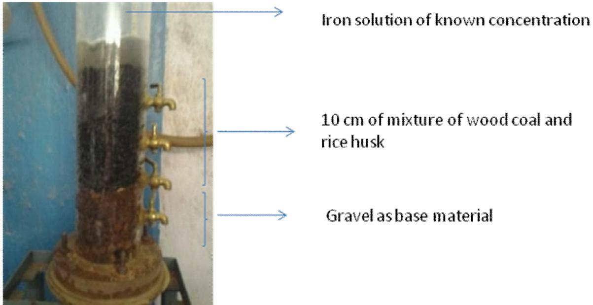
Fig 4.4 Filtration using wood charcoal and rice husk as adsorption media
