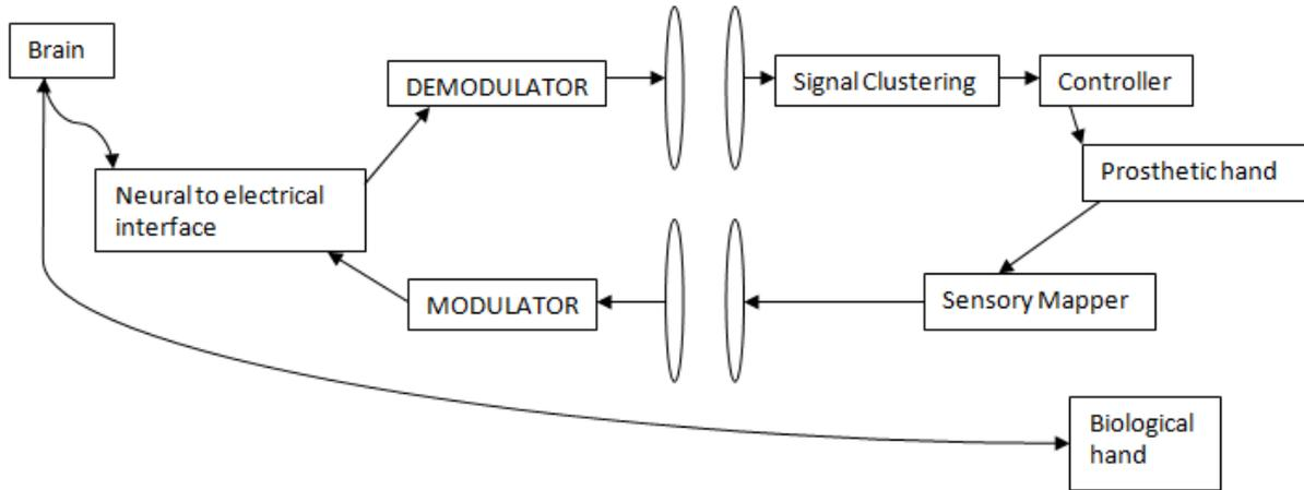
**Figure 2.1: Architecture for using neural networks to control a prosthetic hand (Wan, et al, 1990).**
