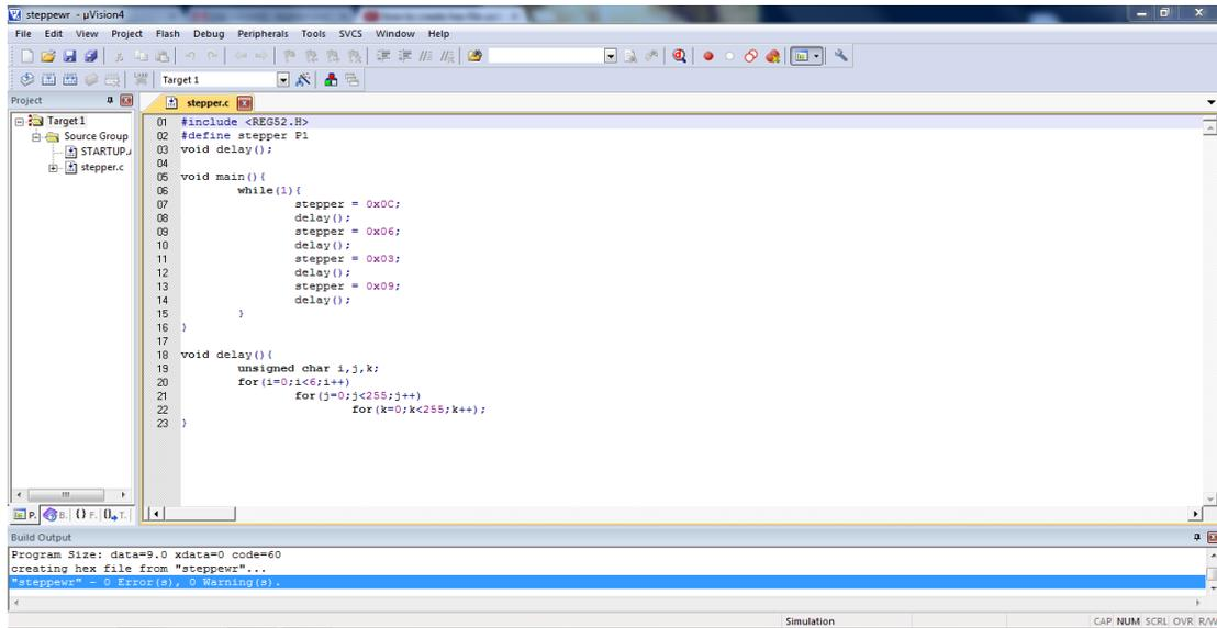
**Figure 4.14 Keil’s µvision IDE Environment and the Code Written For 8052. In The Bottom, It Can Be Seen That An Output Is Printed As “Creating Hex File From “Stepper”... Which Indicated Successful Compilation Of .Hex File to Be Dumped Into the 8052 Microcontroller.**
