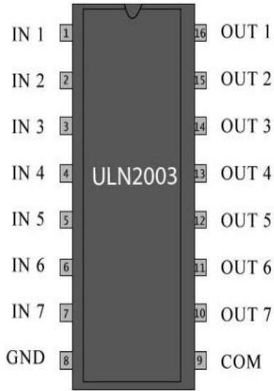
**Figure 4.2: *ULN2003 Pin Diagram.***
