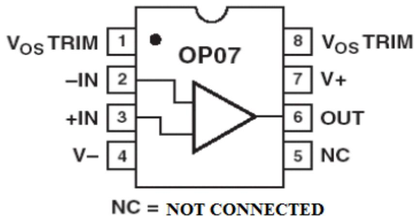
**Figure 4.9: Pin Configuration of Op07**
