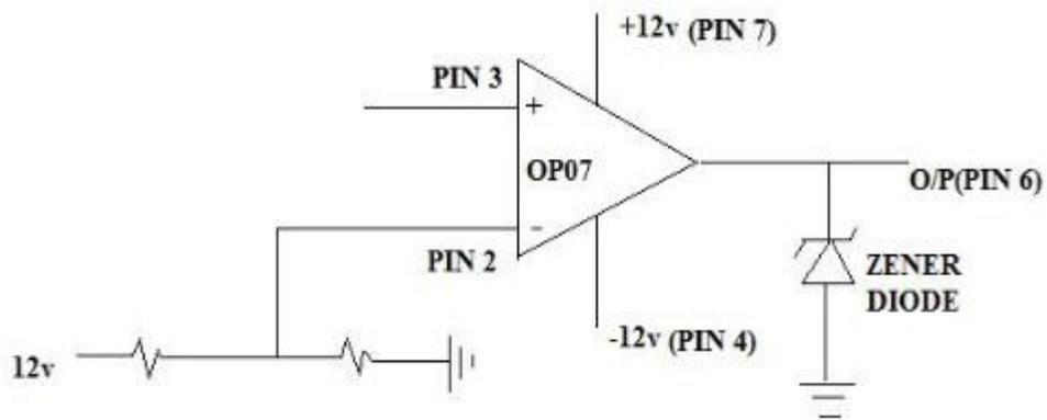
**Figure 4.11: Comparator Using Op-Amp**
