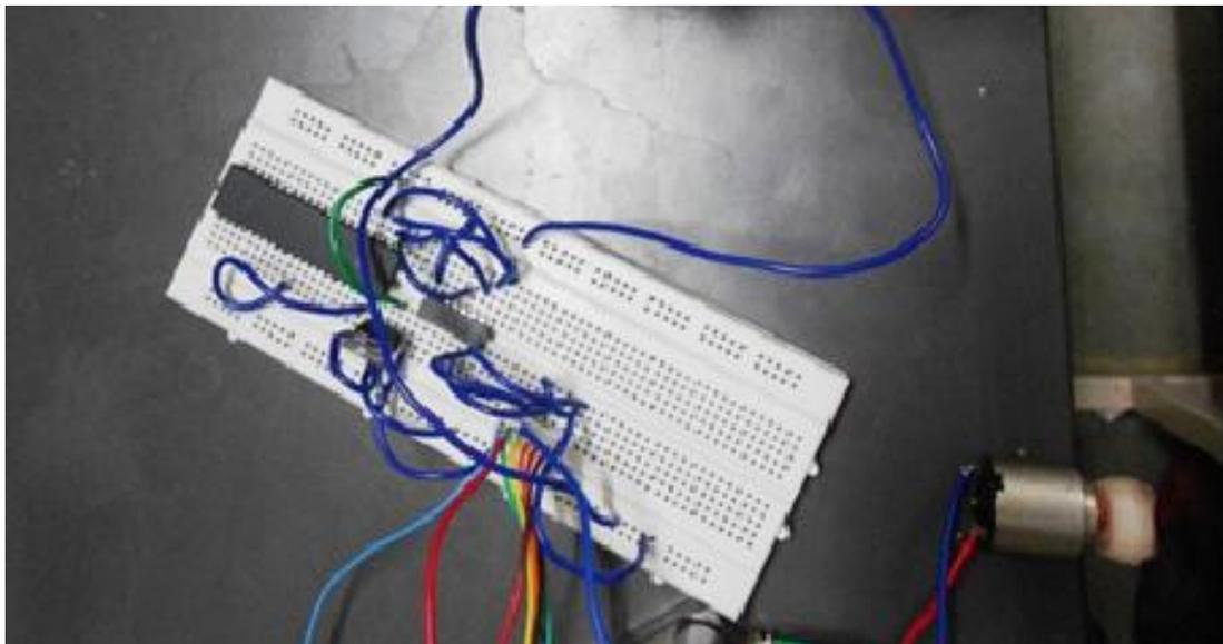
**Figure 4.15 Whole Circuit Diagrams for Motor Control Using Microcontroller and ULN2003.**
