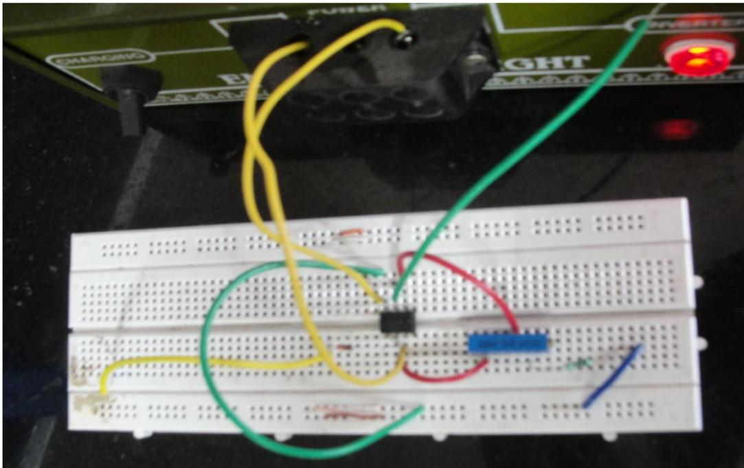
**Figure 4.12: Whole Circuit Diagram for Comparator Using Op-Amp (Op07)**
