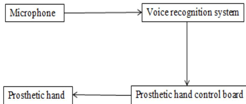
**Figure 2.4: Architecture for Controlling Hand Prosthesis (Mainardi Et Al, 2007).**
