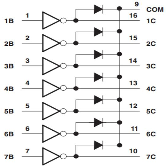
**Figure 4.3: *ULN2003 Logic Diagram.***
