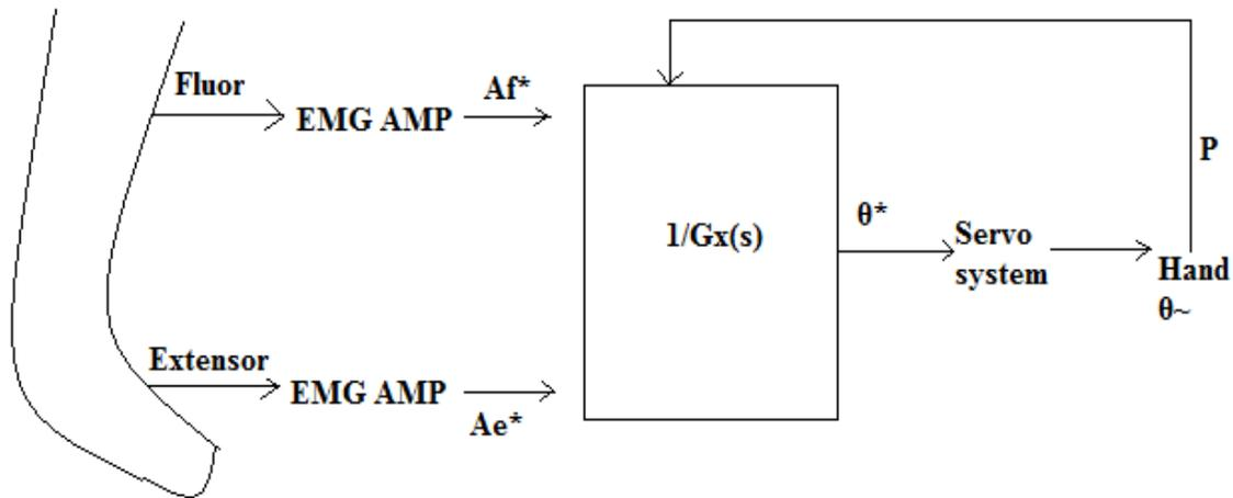
**Figure 2.2: Architecture Block Diagram of the Prosthetic Hand (Akazawa Et Al, 1996).**
