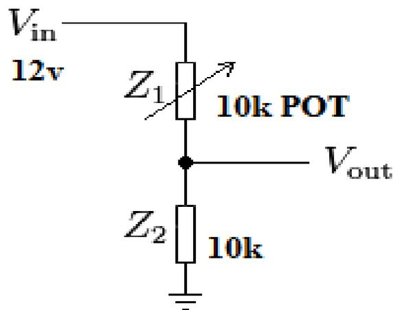
Figure 4.10: Diagrams for Voltage Divider Circuit.
