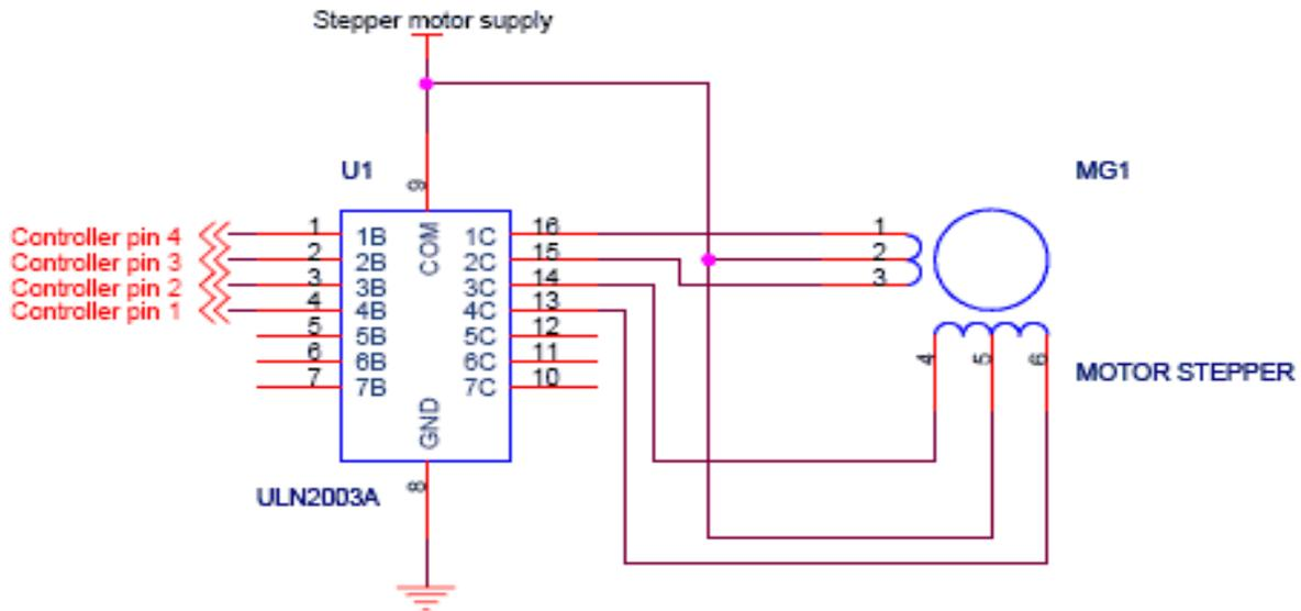
**Figure 4.13: Circuit Setup for Driving Motor Using ULN2003A And Microcontroller.**
