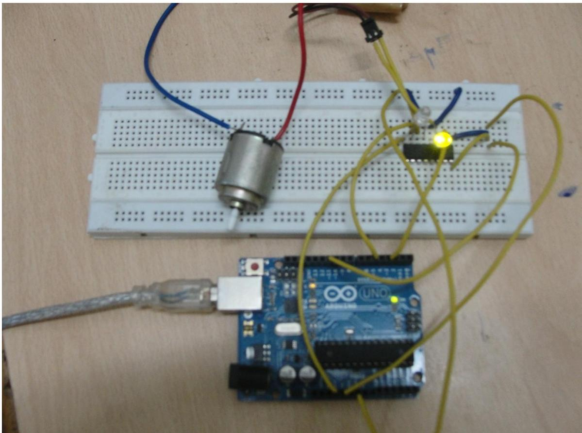
**Figure 4.17: The Whole Circuit Diagram for Motor Control Using Arduino and L293D.**
