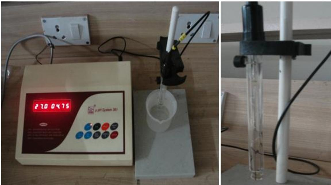
**Figure 4.7: pH Meter and Glass Electrode**
