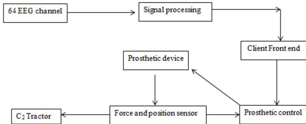
**Figure 2.3: Experimental Setup Used By (Murguialday Et Al, 2007)**
