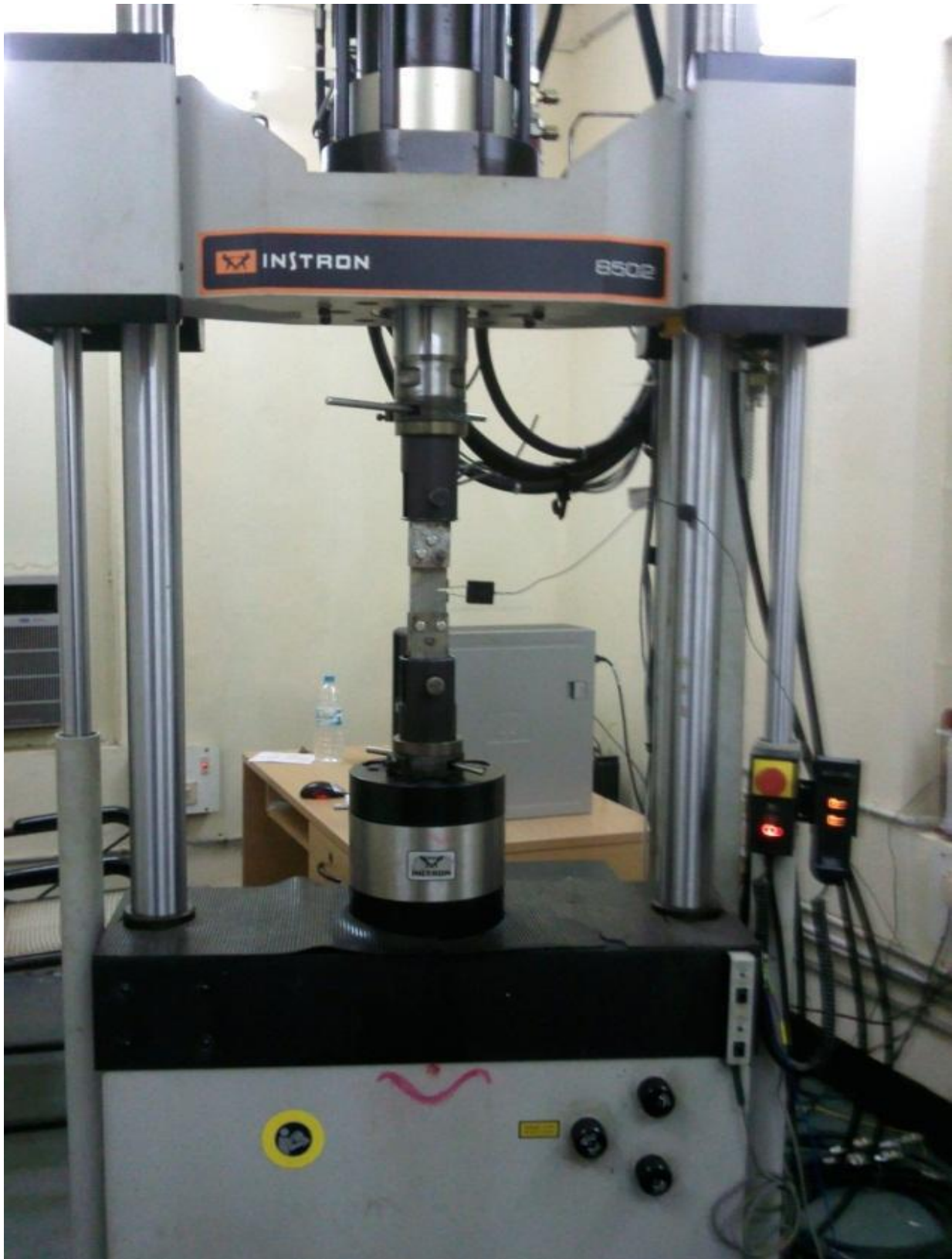
Fig.2. Instron 8502 with SENT specimen
