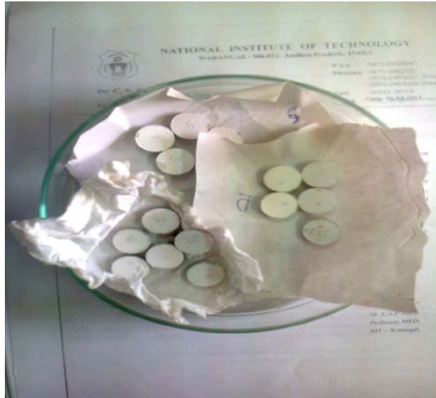
Figure 4.2 Image of sintered pellets
