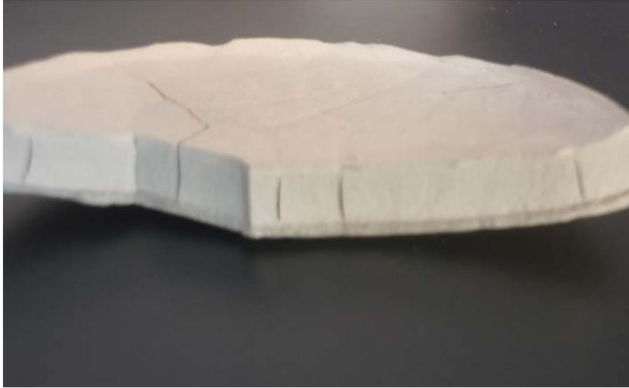
Fig. 4.5 Composite made of gelcasting in conventional way.
