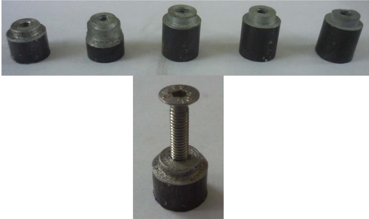
Fig. 4.18: Machinable sintered product prepared through powder metallurgy process.
