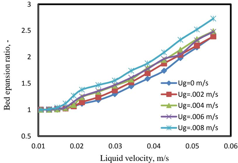
Fig.3.7. Variation of bed expansion ratio with liquid velocity for different values of gas velocity at [Hs = 0.23 m, dp = 3.7 mm]
