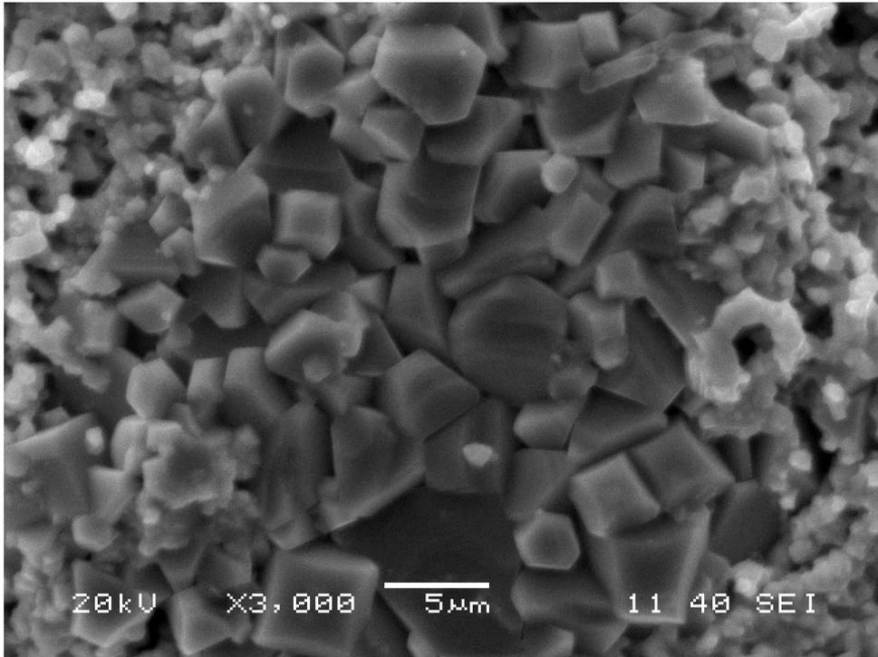
Figure 10 (c). shows the microstructure of .6BT-.4CF composition
