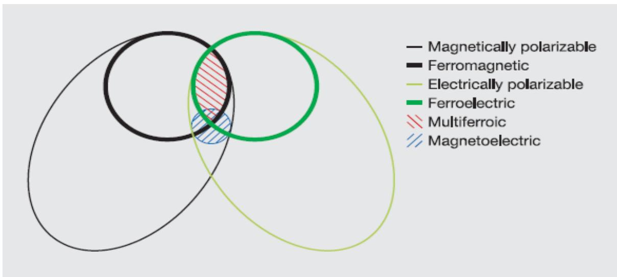
Fig1-The relationship between multiferroic and magnetoelectric materials.
