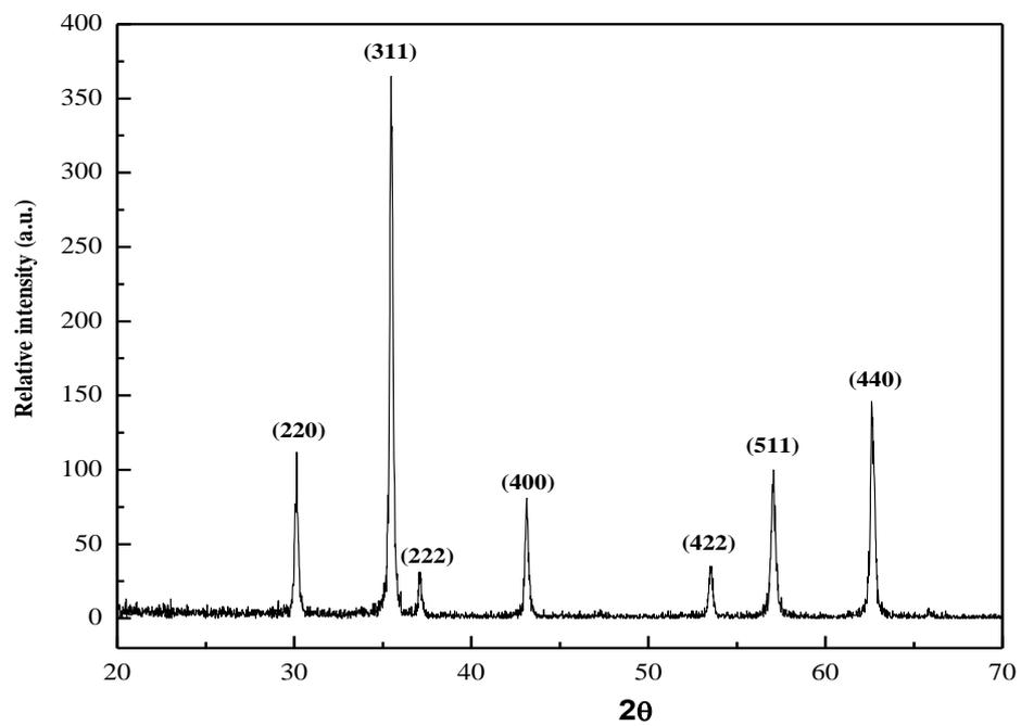
Figure 4.: CoFe<sub>2</sub>O<sub>4</sub> calcined at 900 °C/2h
