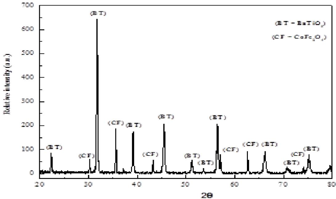
Figure 7.: XRD of 0.6BaTiO<sub>3</sub>-0.4CoFe<sub>2</sub>O<sub>4</sub> composite
