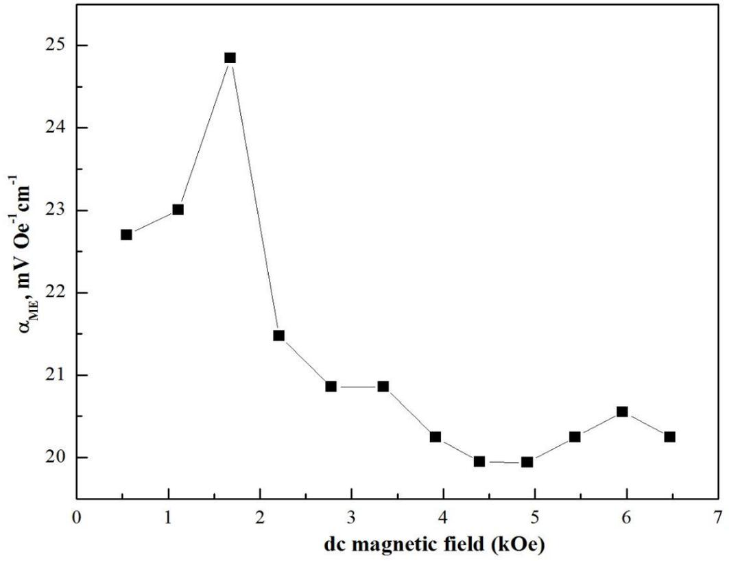
Figure 11 (c). Magnetolectric voltage co-efficient of BTCF composite (BT80% + CF20%)
