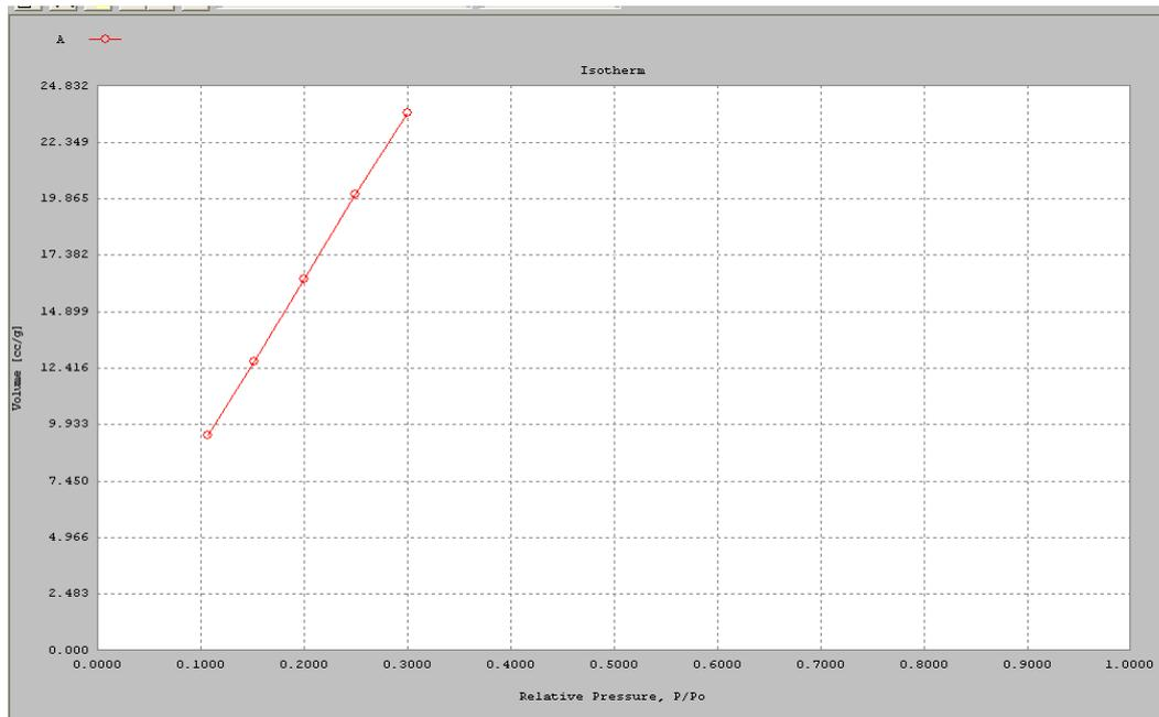
Figure -8 BET surface area of calcined  $\text{CoFe}_2\text{O}_4$  powder
