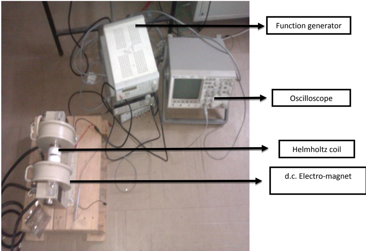
Fig 2. set-up for the measurement of magnetoelectric voltage coefficient.
