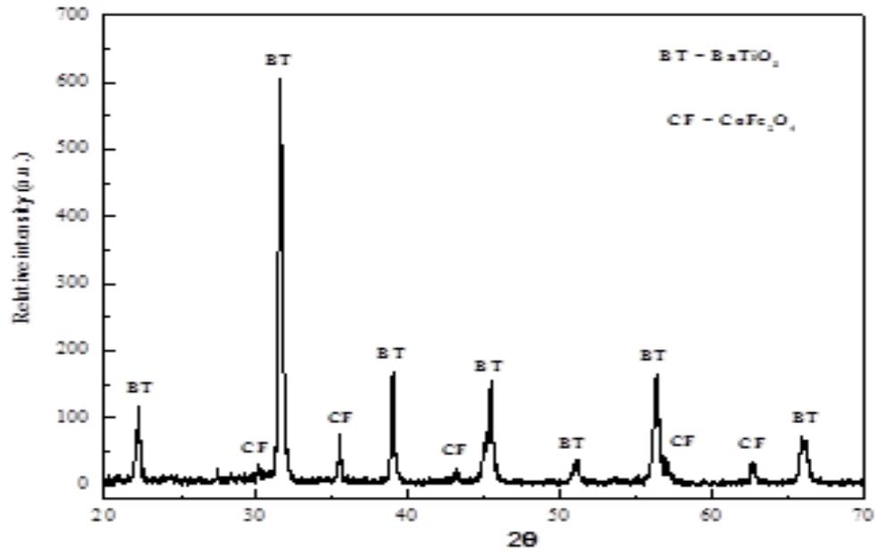
Figure 5.: XRD of mixed BaTiO<sub>3</sub> and CoFe<sub>2</sub>O<sub>4</sub> powder
