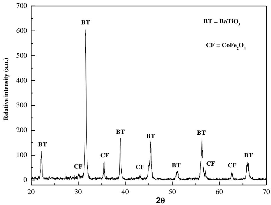
Figure 6.: XRD of 0.7BaTiO<sub>3</sub>-0.3CoFe<sub>2</sub>O<sub>4</sub> composite
