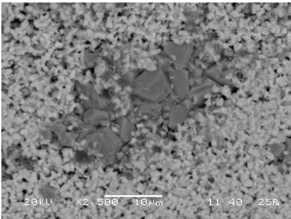
Figure 10 shows the microstructure of .7BT-.3CF composition
