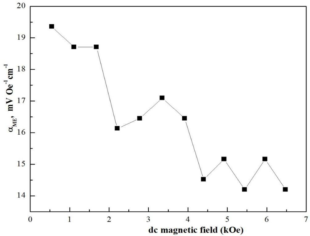
Figure 11 (a). Magnetolectric voltage co-efficient of BT60% + CF40%
