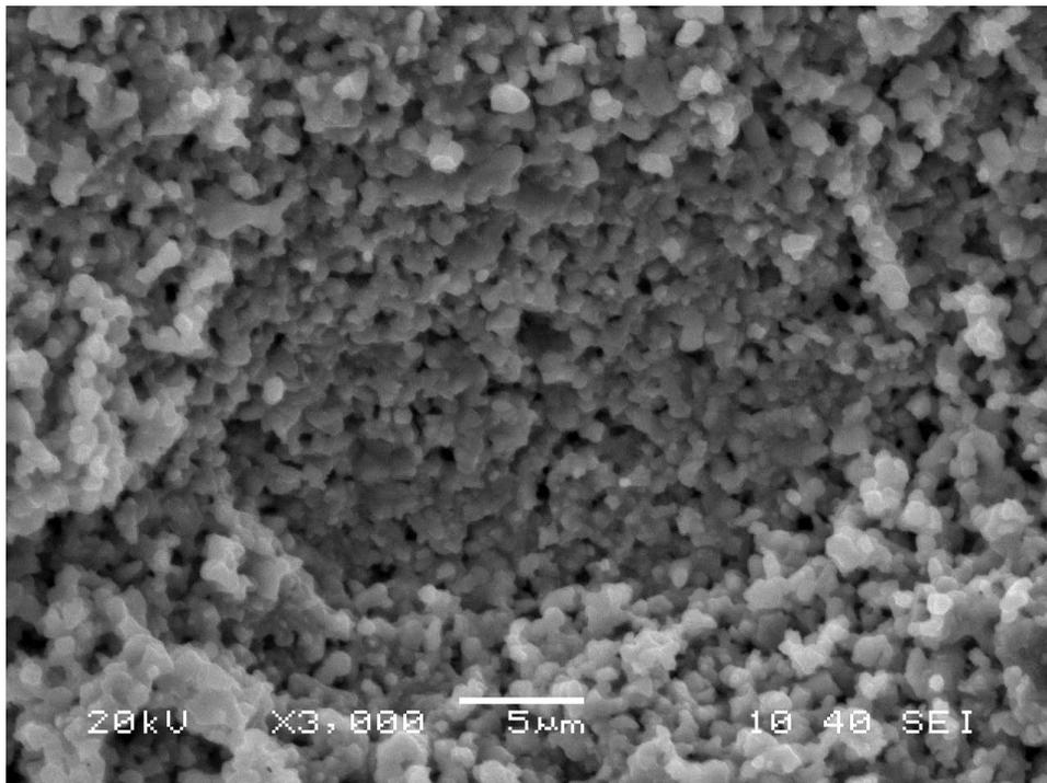
Figure 10 (d)Shows the microstructure of .8BT-.2CF composition
