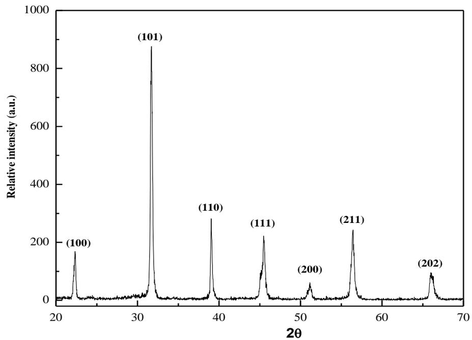
Figure3.: BaTiO<sub>3</sub> calcined at 1000 °C/4h
