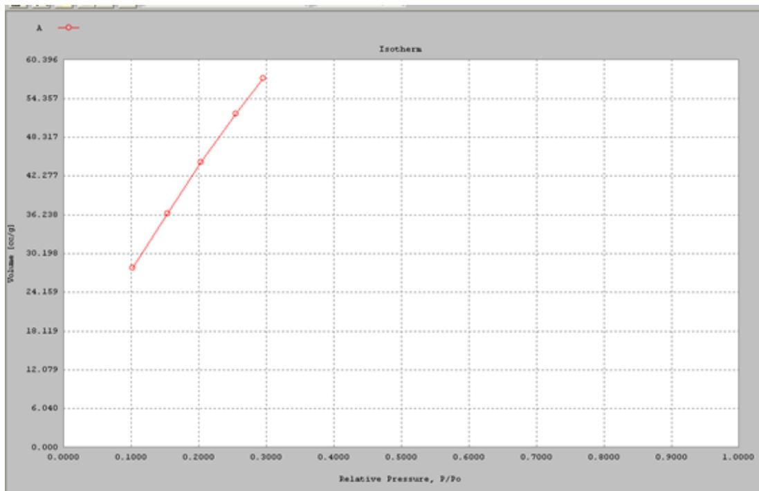
Figure 9. BET surface area of calcined  $\text{BaTiO}_3$  powder
