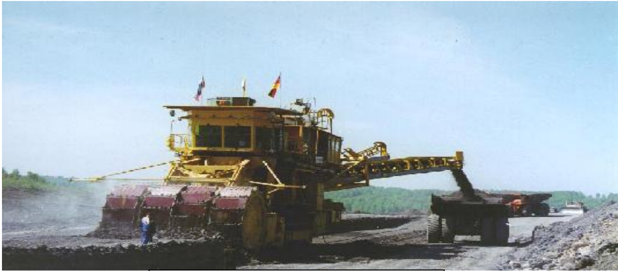
Fig-2.3 Machine with front cutting wheel
