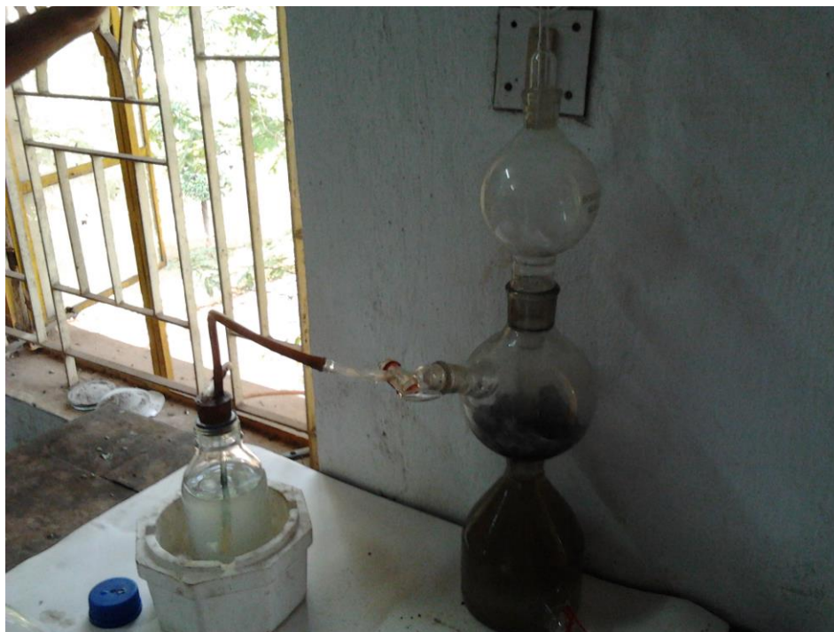
Fig 3.1 Kipp's apparatus set up in lab
