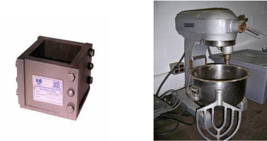
Figure 4: showing 50 mm mould and Hobart mixer
