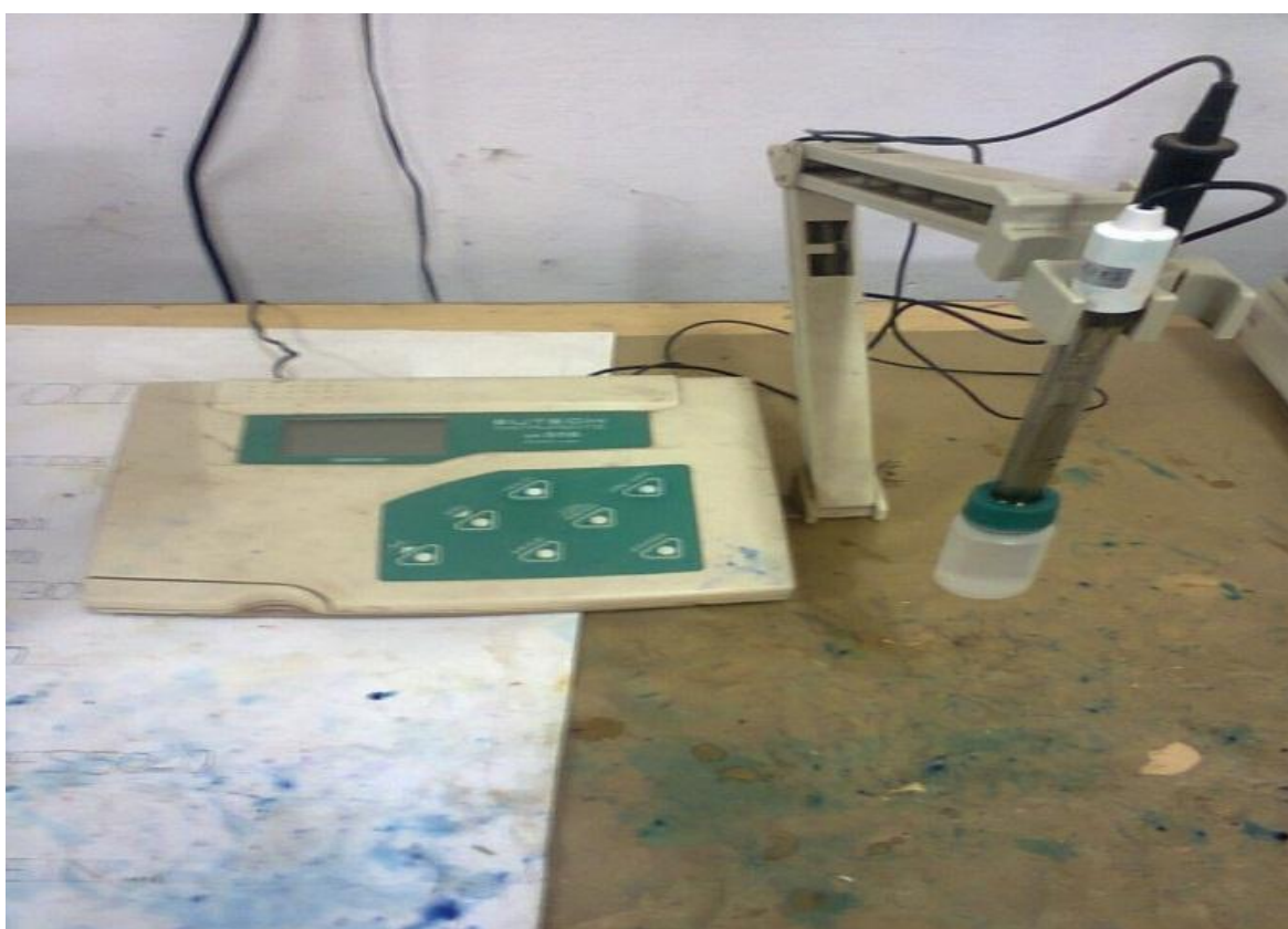
Figure 3 the pH meter used to determine the solution pH
