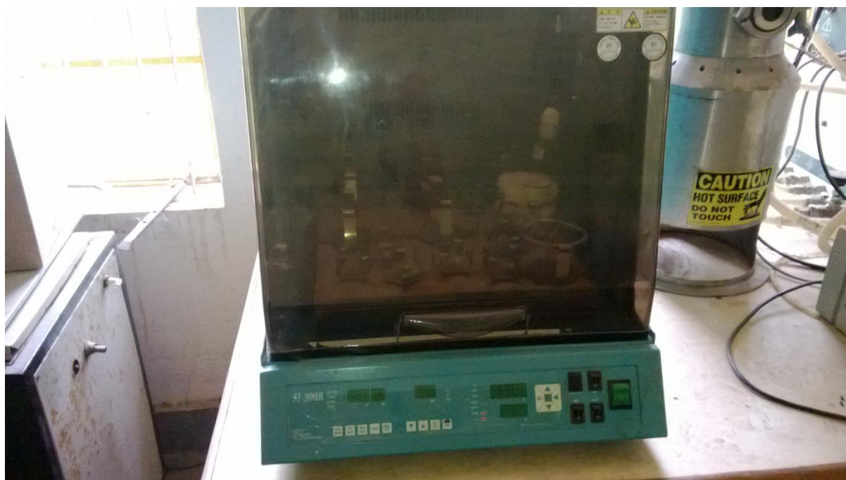
Figure 1 The orbital shaker used for the experiments.
