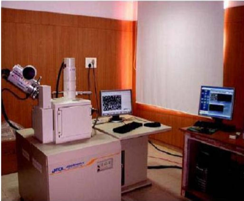
Fig. 4.5 JEOL JSM-6480LV scanning electron microscope
